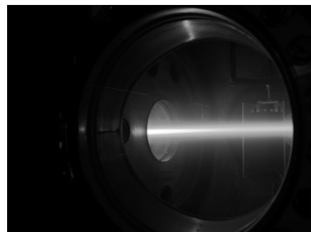
Fig.2 The first MAP-II Plasma in Univ. Tsukuba. Ar plasma 15 A in discharge current (30/Mar/2016).
