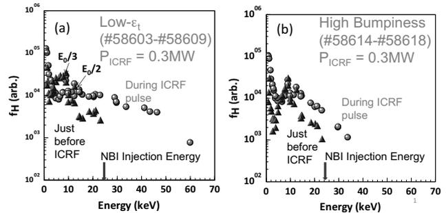
Fig. 1. The measured minority-hydrogen energy spectra of w/ and w/o ICRF pulse for (a) the low- $\epsilon_t$  configuration and (b) the high bumpiness configuration. The target plasma is produced by ECH (0.33 MW) and NBI heating (0.4 MW). The ICRF injection power is 0.3 MW. Measured flux is at the pitch angle of 52°.
