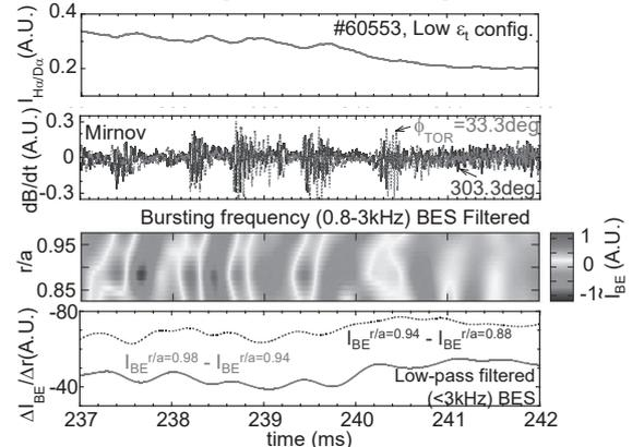
Fig. 2. Time evolution of  $I_{H\alpha/D\alpha}$ , two Mirnov coil signals, band-pass filtered density fluctuation for the burst frequency and difference of low-pass filtered (<3kHz) BES intensity normalized by its distance  $\Delta r$ .
