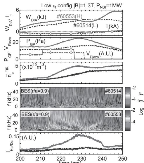
Fig. 1. Time evolution of plasma parameters obtained in H-mode transition (#60553) and no-transition (#60514) plasmas. H-mode transition occurred at  $t = 240$  ms for #60553 with change in the decreasing rate of  $I_{H\alpha/D\alpha}$ .
