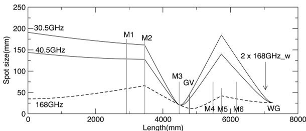
Fig. 2: effective diameters of the quasi optical mirrors (M1-M6) and the beam spot sizes calculated based on the geometrical optics with the use of curvature radii of each mirror
