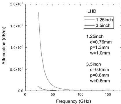
Fig. 1: Power attenuation of the 1.25 inches and 3.5 inches corrugated waveguides use in the LHD ECRH transmission lines.
