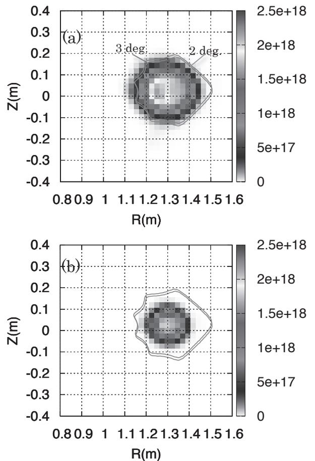
Fig. 1. Density distribution of ions produced by NBI in two loss particle loss boundary cases: (a) vacuum vessel wall and (b) LCFS.
