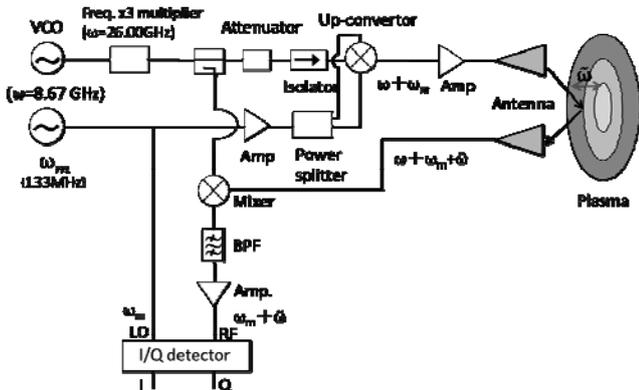
Fig. 1. Schematic of reflectometer system for density fluctuation measurement
