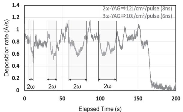
Fig. 2 Lithium aerosol arrival rate data, measured by a quartz crystal film thickness monitor, with and without 2ω-YAG laser beam irradiation, indicated by the yellow-highlighted zones.
