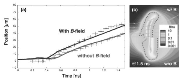
Fig. 1: Trajectory of laser-driven polystyrene foils with and without external magnetic field. Dots and lines are experimental and simulation results. (b) Two-dimensional density profile at 1.5 ns calculated with two-dimensional PINOCO-MHD code. In this experimental condition, the dimensionless parameters are  $\beta > 100$  and  $\chi \sim 1 - 3$  in the corona plasma.
