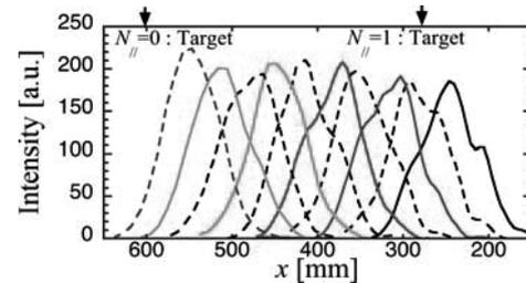
Fig.2: Steering performance tests in toroidally oblique injection-control on the parallel refractive indexes of  $N_{\parallel}$  from zero (i.e. perpendicular injection) to unity (i.e. tangential injection).
