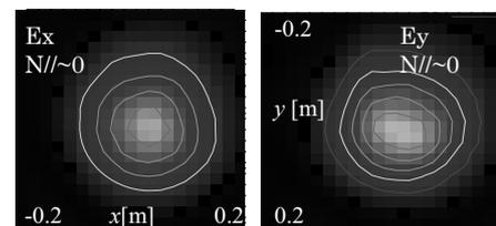
Fig.3: Beam patterns of horizontal and vertical wave-fields of  $E_x$  and  $E_y$  in the perpendicular injections.
