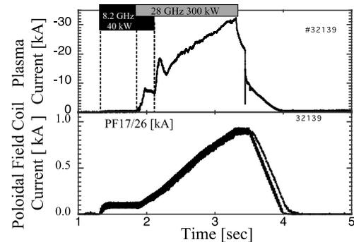
Fig.4: Time evolution of the plasma current and poloidal field coil current. The 30 kA plasma was started up and ramped up by the 140 kW optimized oblique injection, following the poloidal magnetic field ramp-up.
