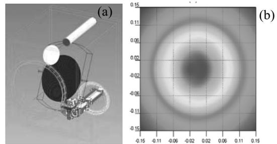
Fig.1 (a): A schematic of the 28 GHz launcher system. The radiated wave from corrugated waveguides was led to the 2<sup>nd</sup> large focusing mirror by the 1<sup>st</sup> convex mirror. The 8.56 GHz components in the hybrid launcher system are also shown in the figure. (b): A evaluated beam pattern at the resonance using a 3D electromagnetic simulator. A strongly focused beam with a diameter of  $\sim 0.01$  m was evaluated along the design.
