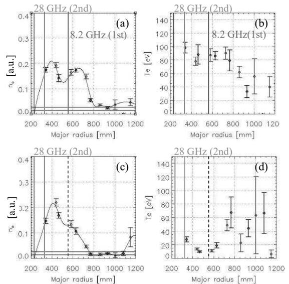
Fig. 2 Electron density (a), (c), and temperature (b), (d) profiles for the initial phase (Figs. (a) and (b)) and the second phase (Figs. (c) and (d)).
