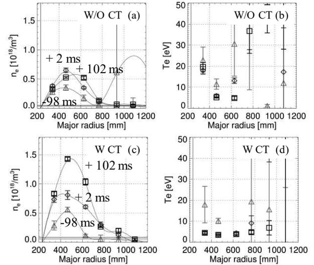
Fig. 1 Electron density (a), (c), and temperature (b), (d) profiles for the cases without and with CT injection. Triangles, diamonds and squares represent the profiles at -98, +2 and +102 ms from the CT injection timings, respectively.
