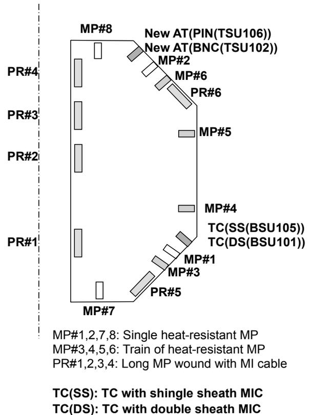
Fig. 1. The location of the magnetic sensors with poloidal cross-section of the vacuum vessel of QUEST. New AT probes and TC probes are installed at the same poloidal position of the other same types of probes. MP#3, #4, #5 and #6 are original AT probes.
