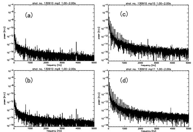
Fig. 2. Power spectral density of the magnetic sensor signals in 8.2 GHz RF heated plasmas. (a) TC probe with double sheath, (b) TC probe with single sheath, (c) New AT probe with multi-pin feed through (d) New AT probe with BNC feed-through.
