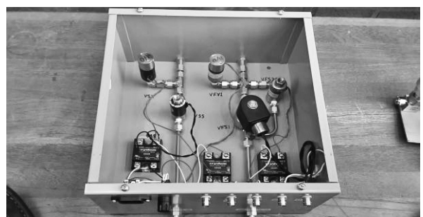
Fig. 2: Control box for activating one gas valve. Not shown here are the trigger system and the fast valves.
