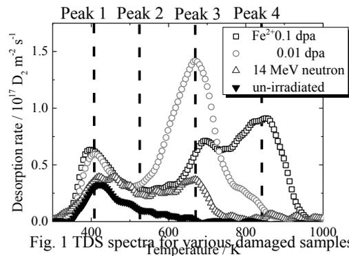
Fig. 1 TDS spectra for various damaged samples
