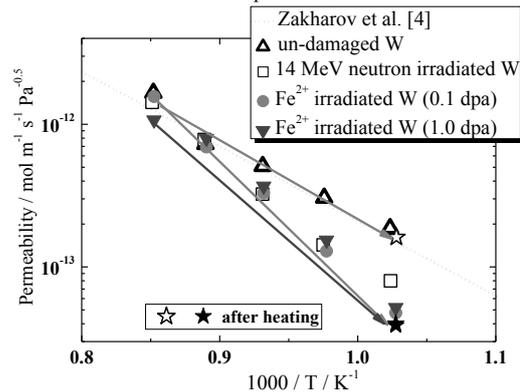
Fig. 2 D permeabilities for Fe<sup>2+</sup> irradiated W and neutron irradiated W, as compared with un-irradiated W and other experimental result.
