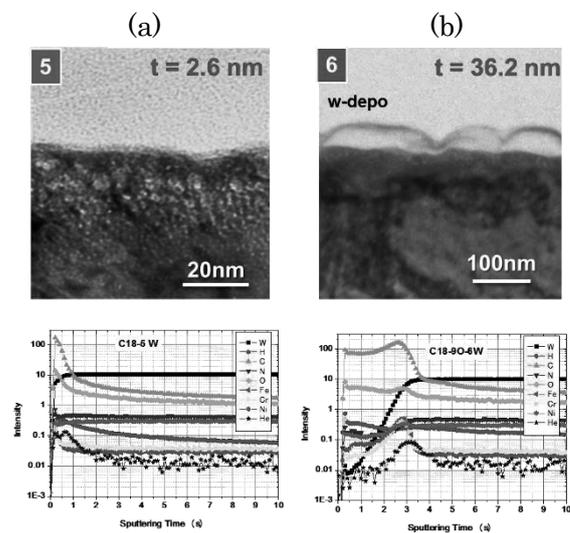
Fig.2 Cross-sectional TEM images of SUS316L and depth distributions of elements in W. (a): Position 5 in erosion dominant area, (b): Position 6 in deposition dominant area.
