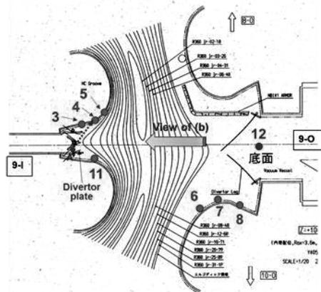
Fig. 1 Position of the coupons from 3 to 13
