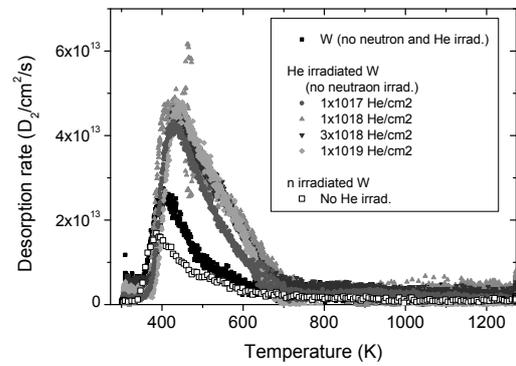
Figure 1 Thermal desorption spectra of D<sub>2</sub> in only He pre-irradiated W and in both neutron and He pre-irradiated W.
