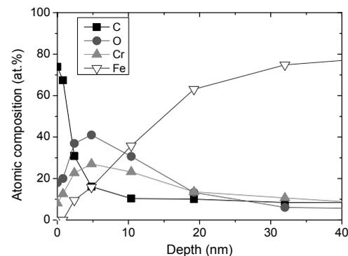
Figure 3 Depth profile of atomic composition in F82H before ion irradiation.
