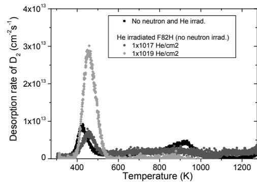
Figure 2 Thermal desorption spectra of D<sub>2</sub> in He pre-irradiated F82H.
