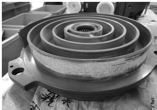
Fig. 13. White dust of the inner scroll.
