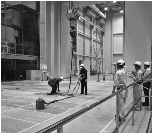
Fig. 18. Transport test of storage vessel.
