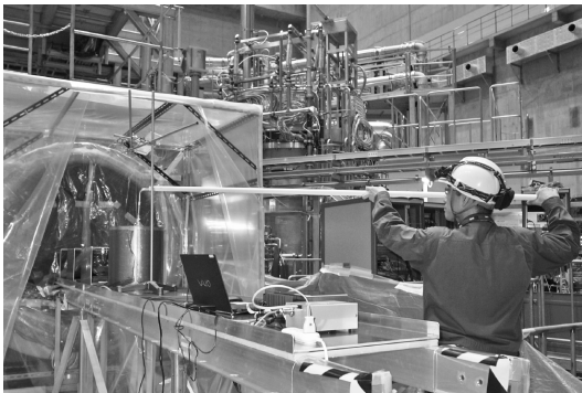
Fig. 19. Moving test of the source using a hook-up tool from the storage vessel to the movable body.
