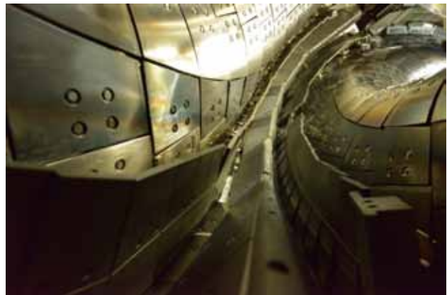
Fig. 4 Photograph of the divertor in which the improved cryo-sorption pump is installed.
