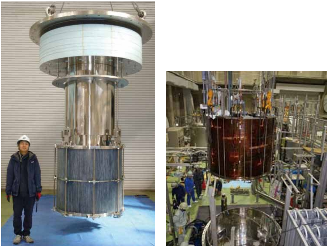
Fig. 2 (Left) The 13-T solenoid at NIFS. (Right) Installation work of the JT60-SA CS module coil into the experimental facility at the NIFS Superconducting Magnet Laboratory.
