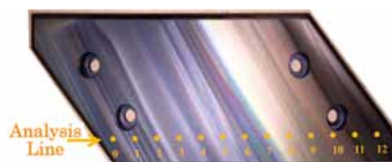
Fig. 3 An LHD divertor tile analyzed by ex-situ LIBS (by Dr. D. Nishijima of UCSD).
