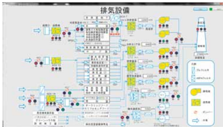
Fig. 13 The exhaust plant monitoring software
