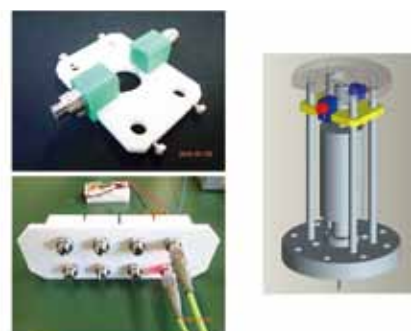
Fig. 3 The parts shielded against a strong neutron using an optical cable.
