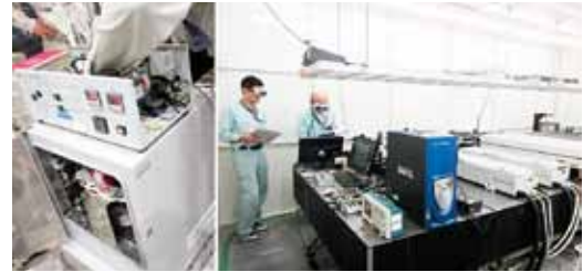
Fig. 12 Maintenance of a methanol supply unit for FIR and operation of YAG lasers for Thomson scattering diagnostics.
