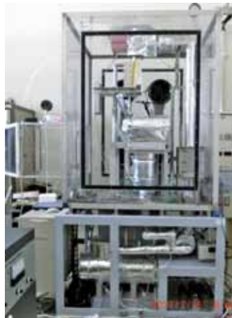
Fig. 11 Experimental setup for investigating the free fall characteristics of liquid metals. Magnetic field is applied to the liquid metal flow using an array of permanent magnets.
