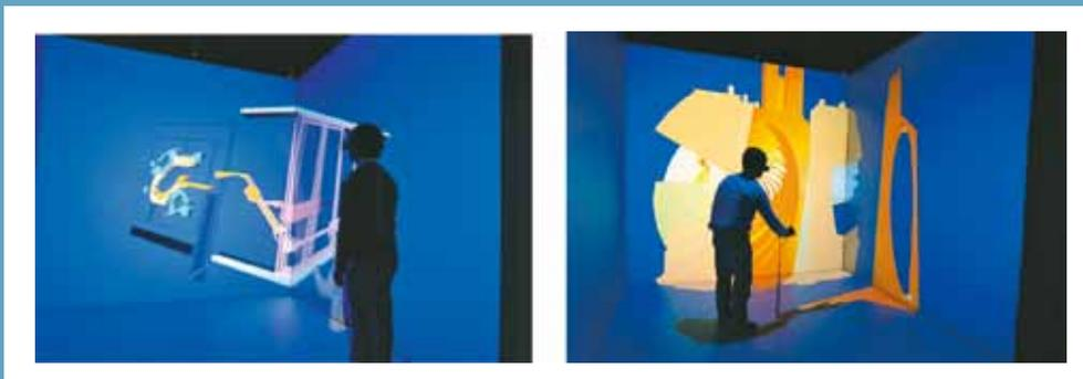
Fig. 1 Virtual-reality visualization of cartridge-type helical reactor CAD data. Left figure shows the reactor design data with robot-arm system, and right figure displays that one component is grasped by the virtual hand.
