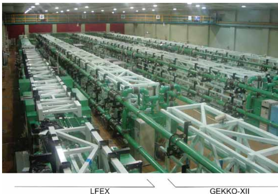
Fig. 2 View of amplifier chains of LFEX and GEKKO-XII lasers.
