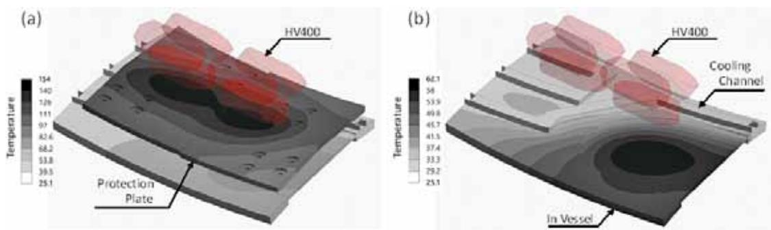
Fig. 7 Temperature profiles of (a) protection plates and (b) in vessel
