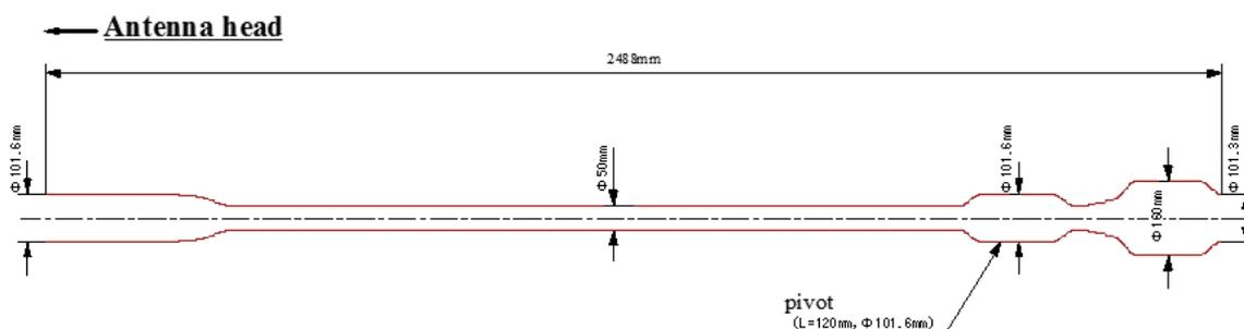
Fig. 8 The design of impedance transformer for HAS antenna
