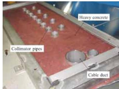
Fig. 14 Multichannel collimator unit made by heavy concrete
