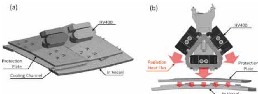
Fig. 6 (a) Model geometry and (b) schematic view of heat flux due to the radiation heating
