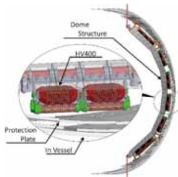
Fig. 5 Geometry of the pumping system using Saes getter NEG pump modules. These modules are connected to the cooling pipe of the dome structure by the support structure.
