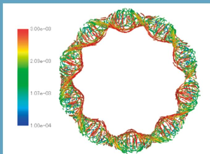
Fig. 1 3D profile of the stream lines of the global flow corresponding to the 1D experimental data.
