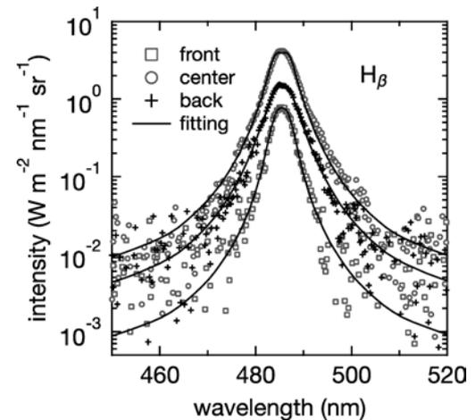
Fig. 3 Fitting results of the observed  $H_\beta$  line at different locations in the ablation cloud. The  $n_e$  at the front edge, center, and back edge are determined to be  $1.2 \times 10^{23} \text{ m}^{-3}$ ,  $1.5 \times 10^{23} \text{ m}^{-3}$ , and  $1.3 \times 10^{23} \text{ m}^{-3}$ , respectively (cited from [2]).
