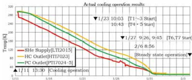
Fig. 15 Actual results of the cooling operation
