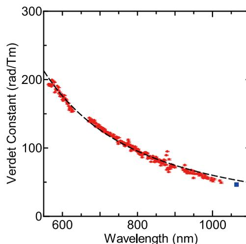
Fig. 3 Verdet constant of Ho<sub>2</sub>O<sub>3</sub> ceramics as a function of wavelength. Cited from Ref. [4].
