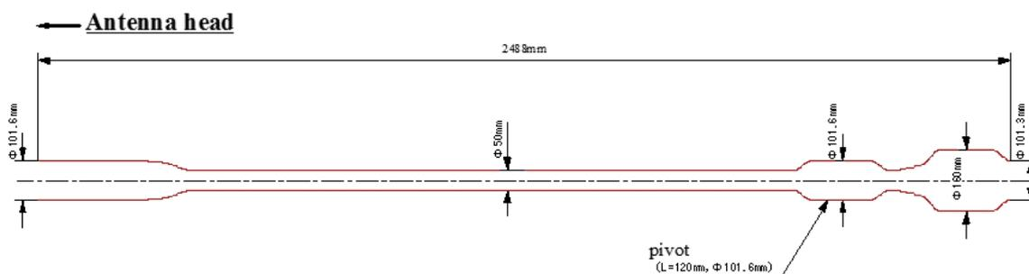
Fig. 8 The design of impedance transformer for HAS antenna
