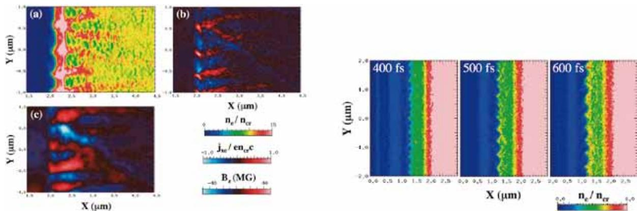
Fig. 2 Left: Weibel structure in the case of relativistic laser intensity at  $t = 250$  fs. (a) electron density, (b) electron current density in X direction and (c) magnetic field in Z direction. Right: Time evolution of electron density profile in the case of non-relativistic laser intensity.
