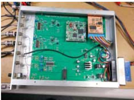
Fig. 1 Phase detection circuit
