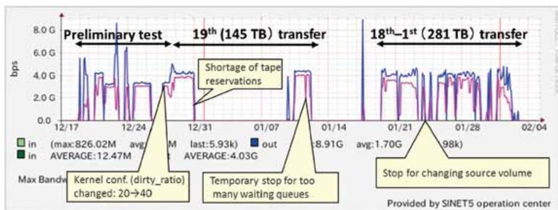
Fig. 2 Network traffic during the LHD → REC full data replication test.
