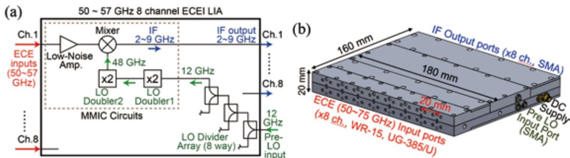
Fig. 1 (a) Schematic diagram of LIA circuit, and (b) outside drawing of LIA.
