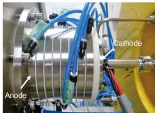
Fig. 2 TPD plasma source for plasma window.
