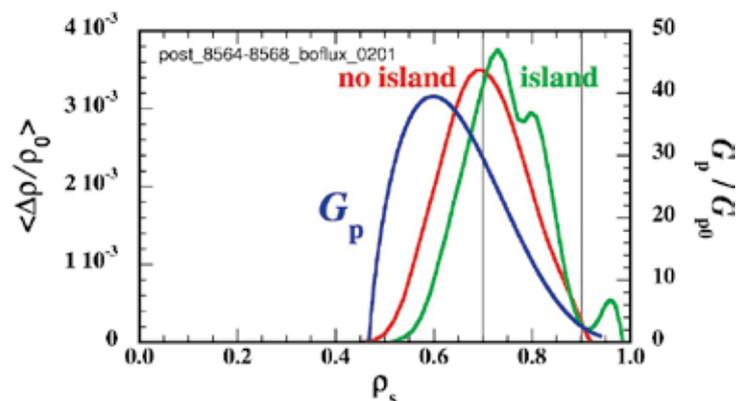
Fig. 3 Normalized plasmoid densities averaged on the flux surface  $\langle \Delta p / \rho_0 \rangle$  as a function of the minor radius  $\rho_s$  with the Boozer coordinate. The red and the green lines indicate those plasmoid densities in the plasmas without and with the islands, respectively. The blue line indicates the normalized ablation rate  $G_p / G_{p0}$ .
