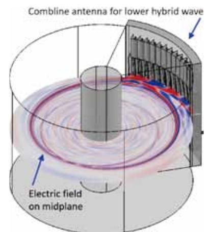
Fig. 1 Electric field distribution on midplane of TST-2. Lower hybrid wave is launched from the comblin antenna.
