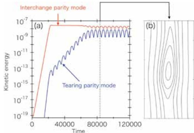
Fig. 2 (a) Time evolution of kinetic energies of both parities of the  $n=1$  mode and (b) magnetic flux surfaces at the final saturated state.
