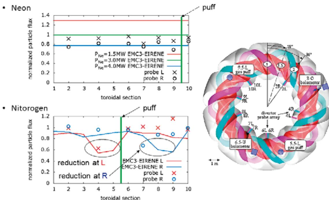
Fig. 2 Configurations of the puffing nozzles, the bolometer systems, and the divertor probe arrays in the LHD and the toroidal flux distribution of hydrogen ions for neon and nitrogen seeding cases.
