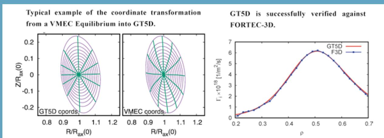
Fig. 1 Coordinate system and the numerical verification of the neoclassical transport in GT5D [1].
