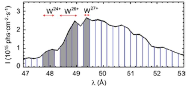
Fig. 2 Tungsten spectrum with UTA lines between  $\lambda = 47 \text{ \AA}$  and  $53 \text{ \AA}$ . The three wavelength intervals indicated by the grey color are identified to be the UTA from  $W^{24+}$ ,  $W^{26+}$ , and  $W^{27+}$  ions, respectively (cited from [1]).
