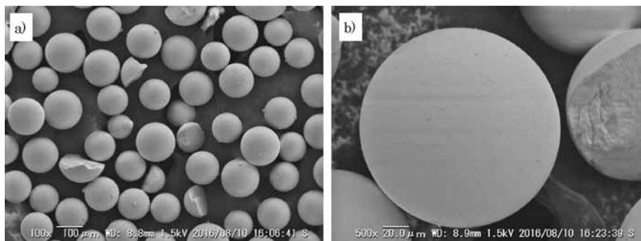
Fig. 15 SEM photo of the cation exchange resin with 90% cross-linkage with two magnifications.
