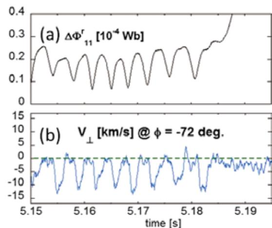
Fig. 1 Temporal change of (a)  $m/n=1/1$  component of the radial magnetic flux and (b) the perpendicular velocity around  $r_{\text{eff}}/a_{99}=0.96$ . Cited from Fig. 3 in [1].
