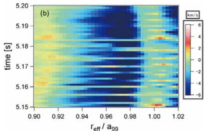
Fig. 2 Spatio-temporal behavior of  $V_{\perp}$  in the plasma edge region. Here,  $r_{\text{eff}}$  is the effective minor radius and  $a_{99}$  is the effective minor radius of which encloses 99% of the total electron pressure. Cited from Fig. 4 in [1].
