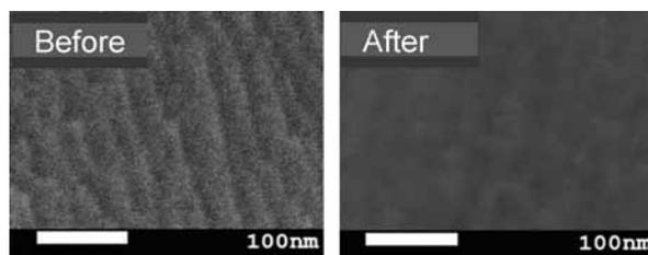
Fig. 8 Surface images of tungsten samples with high heat flux electron beams before (left) and after (right) irradiation by helium ions in the ACT-2 electron-beam facility.
