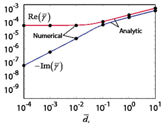
Fig. 3 Growth rates and real frequencies as functions of the ion skin depth obtained numerically from the eigenmode equations (points) compared with the analytic dispersion relation (lines).
