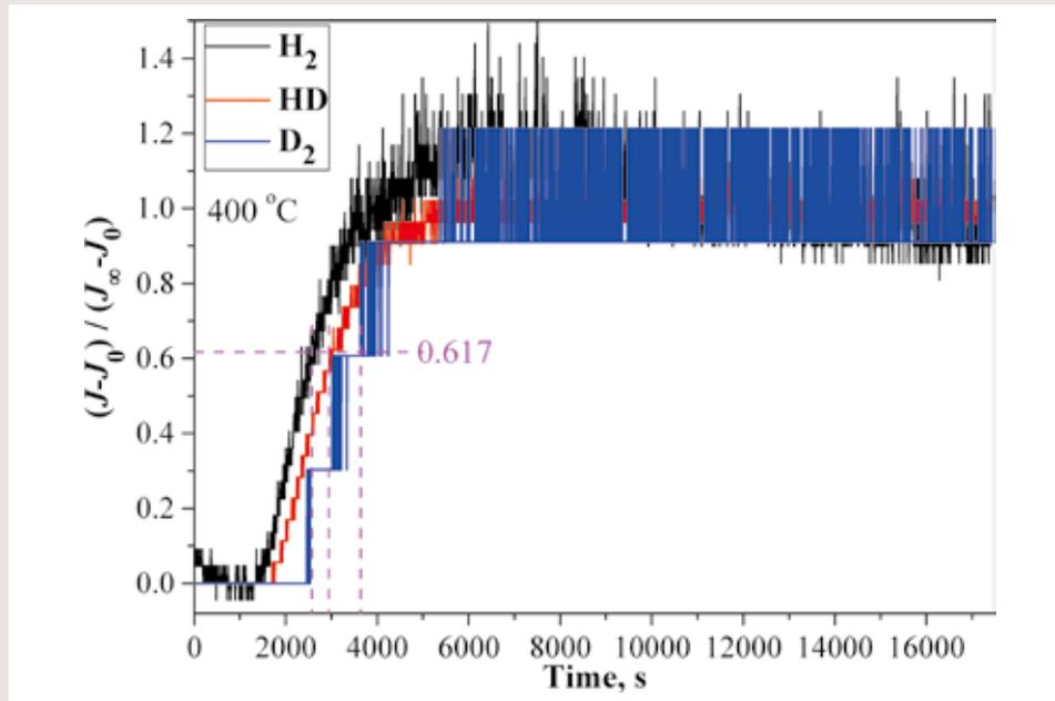
Fig. Permeation curves of H<sub>2</sub>, HD and D<sub>2</sub> under exposure to H<sub>2</sub>-D<sub>2</sub> mixture gas, showing faster diffusion of H than D.
