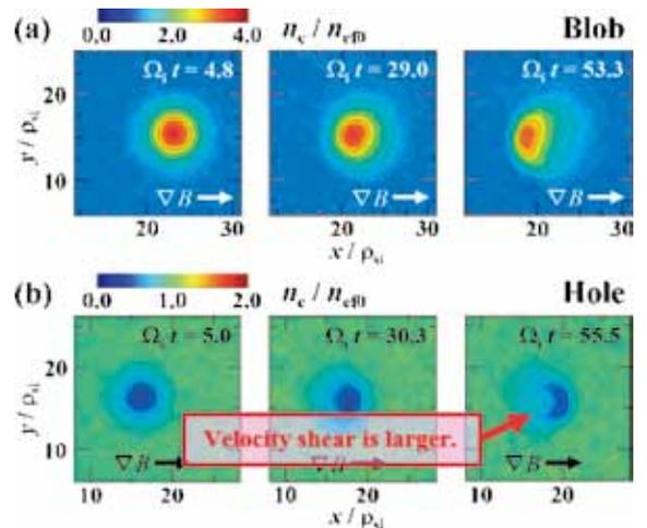
Fig. 2 Time evolutions of the electron density distribution on the poloidal cross-section in the blob (a) and hole (b) propagations. This figure appeared on the front cover of Journal of Plasma and Fusion Research Vol. 93, No. 12 and the top page of the Plasma and Fusion Research website.
