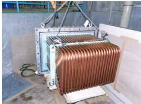
Fig. 11 The lower oil-cooling pipe unit (Removed from a generator)
