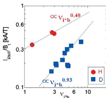
Fig. 1 RMP penetration threshold as the function of the collisionality in the LHD with  $A_p=5.7$  and  $\beta_{\text{local}}\sim 0.3\%$ .
