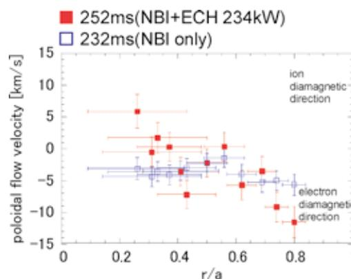
Fig. 2 Poloidal flow velocity profile for NBI+ECH and NBI only plasmas. Balanced injection is made using two opposite tangential beam lines for NBI heating.
