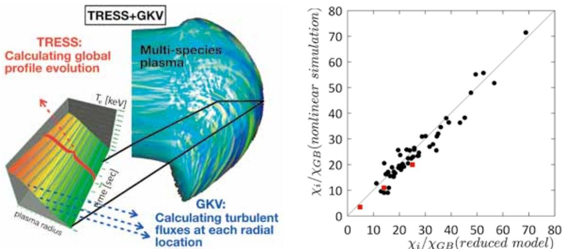
Fig. 2 Left: Joint framework in TRESS+GKV. Multiple local turbulent transport calculations by GKV directly couple to the 1-D global transport solver TRESS.
