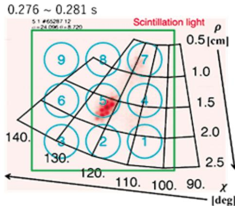
Fig. 3 The observation grid map on the scintillator surface for energy and pitch angle. Blue circles indicate the observation area of each PMT channel. The red part indicate CCD scintillating area observed by a CCD camera.
