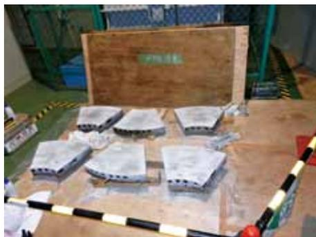
Fig. 12 Penetrant test for thrust metal
