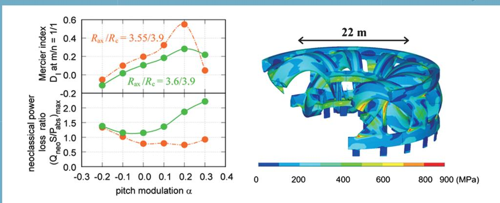
Fig. 1 (left) Dependence of the Mercier index (indicator of MHD instability) and the neoclassical power loss on the pitch modulation parameter  $\alpha$  of the helical coil winding with a different magnetic axis position. (right) The stress distribution on the coil supporting structure in the case of  $\alpha = -0.1$ . The maximum peak stress is within the allowable limit ( $< 1$  GPa).
