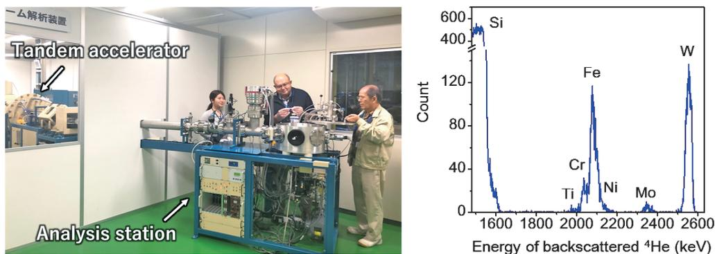
Fig. 6 (left) The ion beam analysis device consisting of an ion beam injector, a tandem accelerator, and an analysis station, and (right) an example of the Rutherford backscattering spectrometry (RBS) spectrum of the mixed-material layers deposited on a Si plate placed inside the LHD vacuum vessel during one experimental campaign.
