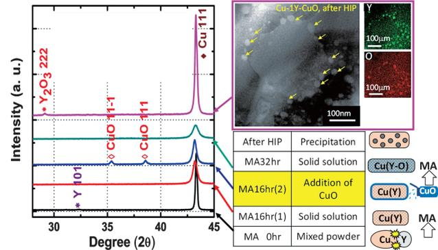
Fig. 3 In-situ fabrication of Cu-Y<sub>2</sub>O<sub>3</sub> alloy.
