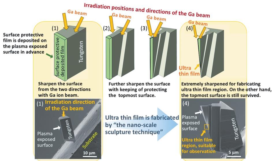
Fig. 4 The “nano-scale sculpture technique” by using a focused ion beam – electron beam (FIB-SEM) device. The upper series shows a schematic view of the fabrication process using a Ga ion beam. The images of (1) and (4) in the bottom series are the corresponding scanning electron microscope (SEM) images to those of (1) and (4) in the upper series.
