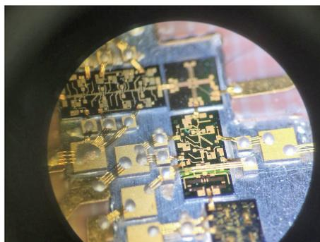
Fig. 4 Wire Bonding
