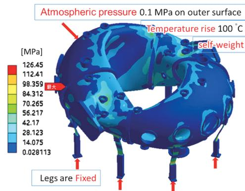
Fig. 6 The stress distribution on vacuum vessel
