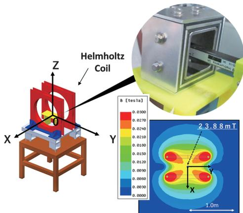
Fig. 5 Arrangement of the Helmholtz coil system, a mockup of magnetic shield, and distribution of magnetic flux density.
