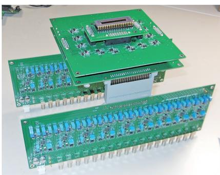
Fig. 3 35ch PIN photo diode amplifier
