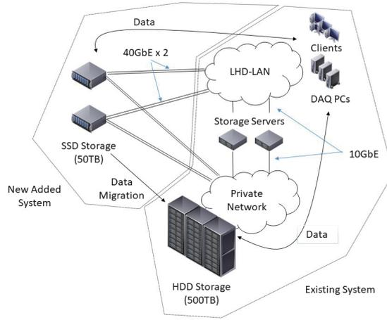
Fig. 15 New DAQ system added SSD storage
