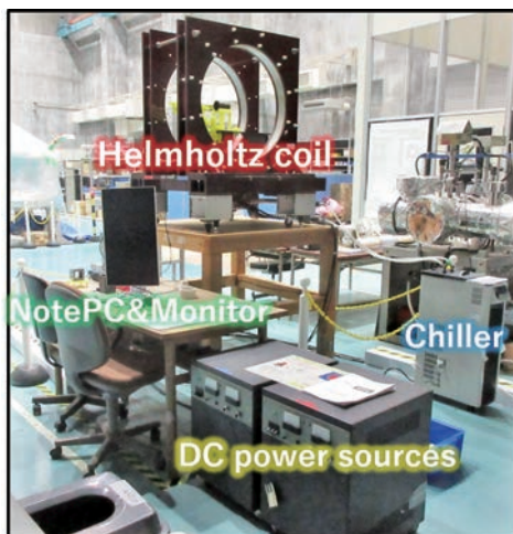
Fig. 20 Overall view of the Helmholtz coil operation system
