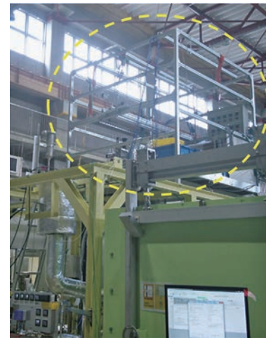
Fig. 3 Expansion of an experimental stage on Oroshhi-2 for the validation experiment of continuous hydrogen recovery from circulated LiPb by the VST technique.
