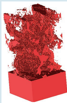
Fig. 1 Tungsten fuzz structure by transmission electron microscopy (TEM. Tecnai Spirit G2, 120 kV, \times 15 k, spot size 6) at the Yasunaga laboratory of Kyushu Institute of Technology. The structure size is 202 nm \times 202 nm \times 530 nm.
