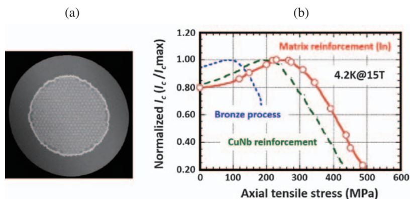
Fig. 11 (a) Typical cross-sectional image of the internally reinforced  $\text{Nb}_3\text{Sn}$  multifilamentary wire. (b) Dependence of the critical current (normalized by each maximum value) on the axial tensile stress for various  $\text{Nb}_3\text{Sn}$  wires.
