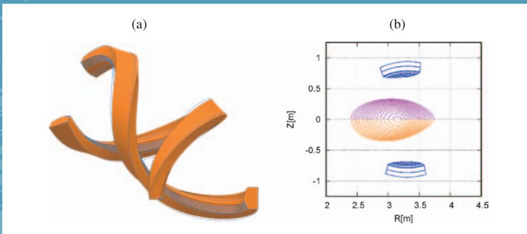
Fig. 1 (a) Variation of the helical winding path with a helical pitch modulation parameter  $\alpha$  of 0.1 (blue dotted-curves) and 0.0 (orange block). (b) Cross-sectional shape of the magnetic surfaces (calculated by the HINT code with a peak beta value of 3%) and helical coils at the horizontally-elongated plasma cross-section with a helical pitch modulation parameter  $\alpha$  of 0.1 (upper) and 0.0 (lower).
