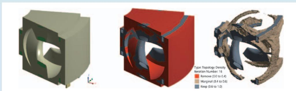
Fig. 14 Example of a design using topology optimization. Left figure is an initial setting, and right one is the optimization result. Red color in the middle figure is the removed region.
