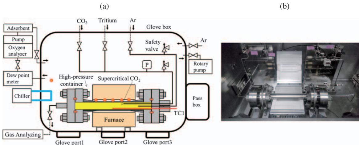
Fig. 15 (a) Design of Supercritical CO<sub>2</sub> gas facility. (b) Photograph of supercritical CO<sub>2</sub> gas facility.
