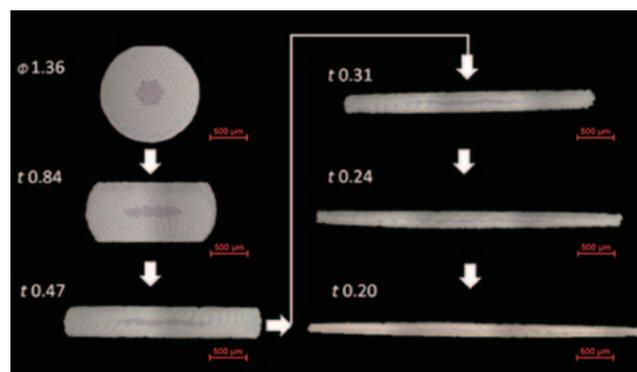
Fig. 16 Fabrication procedure of the tape-shaped RHQT Nb<sub>3</sub>Al conductor (final thickness  $t = 0.20$  mm) starting from a wire-shaped conductor (diameter  $\phi = 1.36$  mm).
