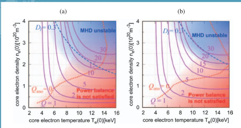
Fig. 2 Comparison of the achievable operation region (the white area without shades) in the diagram of core electron temperature and core electron density for cases of (a)  $\alpha = 0.1$  and (b) 0.0.
