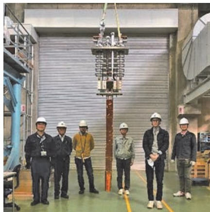
Fig. 11 Experimental setup of the STARS conductor sample to be installed into the NIFS superconductor testing facility.
