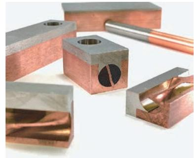
Fig. 4 Bonding samples fabricated using PSB method.
