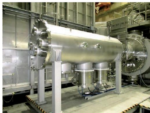
Fig. 5 The additional pumping system with two turbo molecular pumps.
