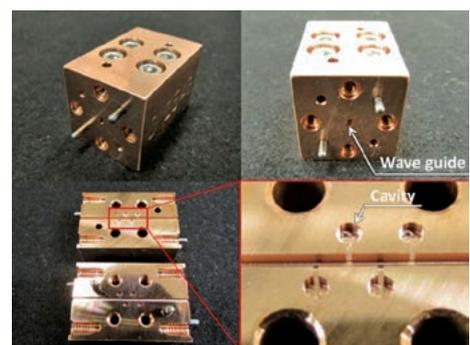
Fig. 2 154GHz Notch filter.
