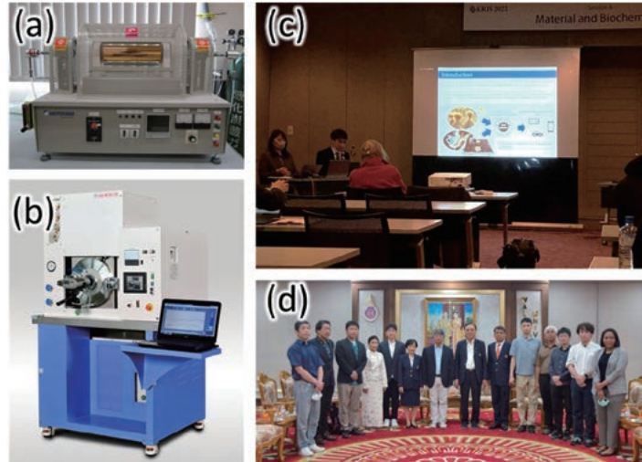
Fig. 13 (a) Rotary kiln device (b) Spark plasma sintering device (c) Presentation in KRIS2023 (d) Group photo at the visit to Warailak University
