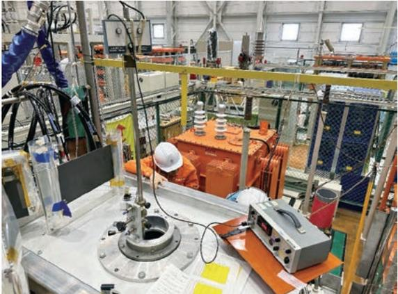
Fig. 1 Magnetic field measurements carried out prior to installation of the gyrotron.
