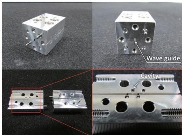
Fig. 1 154 GHz notch filter
