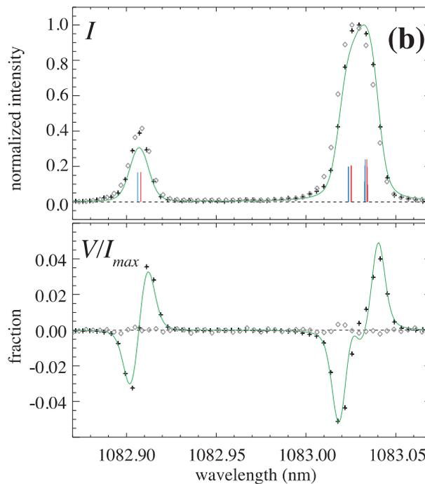
Fig. 4 Normalized intensity  $I/I_{\max}$  and circular polarization  $V/I_{\max}$  from ICP with (black pluses) and without (gray diamonds) magnets under RF power of 100 W and neutral pressure of 5.0 Pa. Blue and red bars show intensities of  $-\sigma$  and  $+\sigma$  components, respectively. Green curves show best fit function. Cited from Ref. [3].
