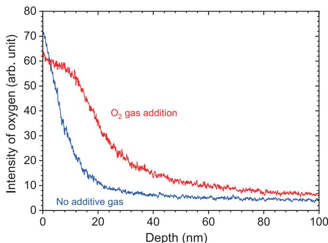
Fig. 2 Depth profiles of oxygen in oxide films formed on Inconel 600 alloy samples by exposing to steam at 280 °C and 6.4 MPa.
