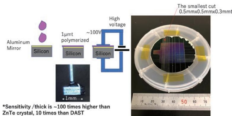
Fig. 3 Process of creation of EO polymer layer on a silicon wafer.
