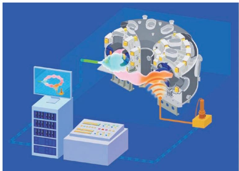
Fig. 1 Image of digital twin control, in which real plasma is controlled by virtual plasma reproduced on a computer.
