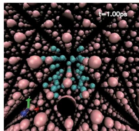
Fig. 5 Snapshot of the atomic structure at 1 ps simulation was performed by randomly injecting 54 hydrogen atoms into a vacancy created by the removal of 9 atoms from a tungsten bcc crystal. The blue and peach balls represent hydrogen and tungsten atoms, respectively.
