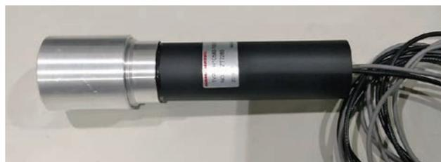
Fig. 2  $\text{LaBr}_3:\text{Ce}$  scintillation detector
