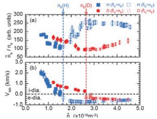
Fig. 1 The line averaged electron-density dependence of (a) the turbulence level and (b) phase velocity of turbulence in the laboratory frame.  $n_{tr}(H)$  and  $n_{tr}(D)$  represent the transition densities in the H and D plasmas, respectively. The blue and red symbols represent the H and D plasmas, respectively. The closed and open symbols represent  $\bar{n}_e < n_{tr}$  and  $\bar{n}_e > n_{tr}$ , respectively. The values are averaged at  $\rho = 0.5-0.7$
