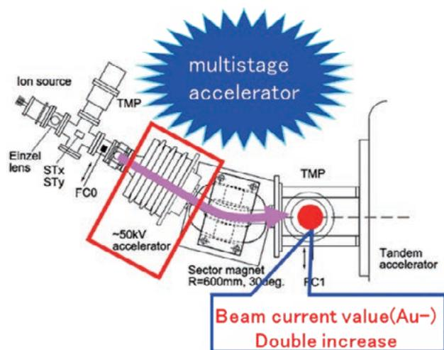
Fig. 9 Beam loss due to multistage accelerator
