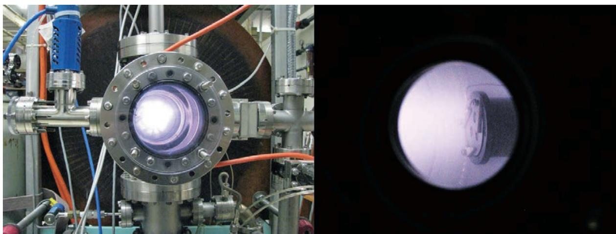
Fig. D+He mixture plasma in DPE and the material samples under the irradiation.
