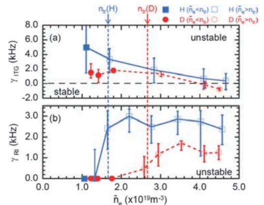
Fig. 2 Electron-density dependence of the linear growth rate of (a) ITG turbulence ( $\gamma_{ITG}$ ) and (b) RI turbulence ( $\gamma_{RI}$ ). The errors in  $\gamma_{ITG}$  and  $\gamma_{RI}$  were evaluated by changing the normalized ion temperature gradient and pressure gradient by 20 %, respectively.
