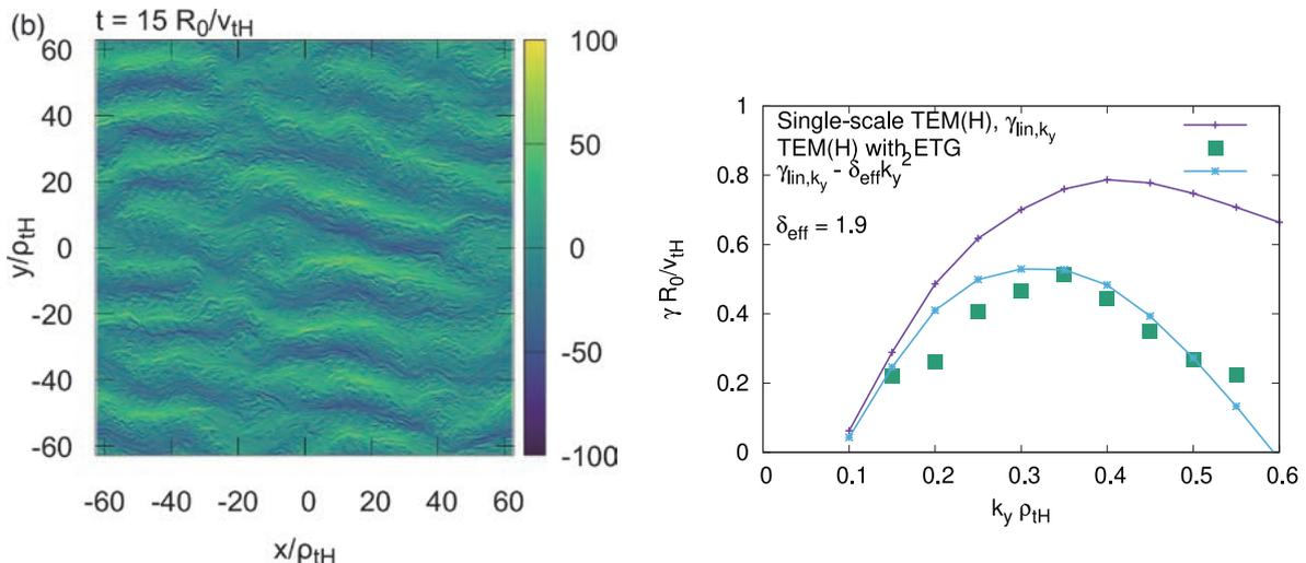
Fig. 1 (left) A snapshot of the toroidal component of an electric field in a growth phase of the trapped electron mode (TEM) in electron temperature gradient turbulence, and (right) growth rates of the TEM instability [1].
