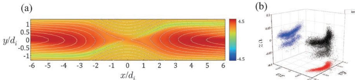
Fig. 7 (a) Magnetic field lines and  $B_z$  (color). Magnetic reconnection is driven in the center. (b) Velocity plots of ion particles as black points. We can see that the 3D structure of a crescent structure is formed in velocity space. Red and blue points are projections into the  $(v_x, v_y)$  and  $(v_y, v_z)$  planes, respectively.
