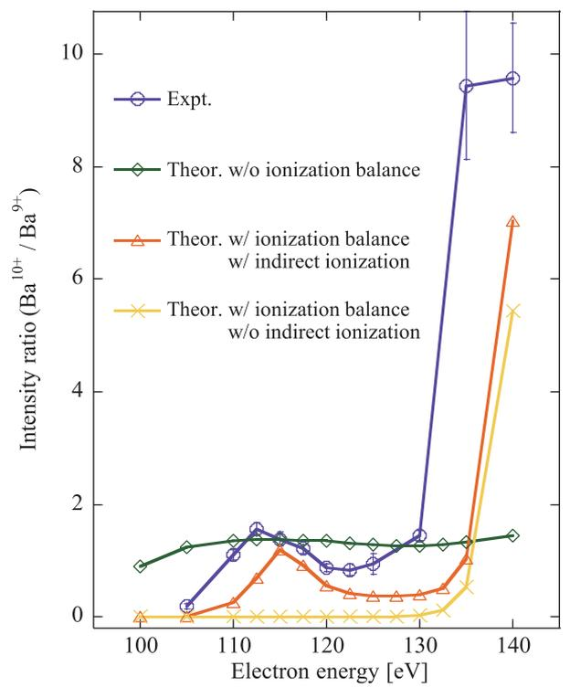
Fig. Electron-energy dependence of the intensity ratio between the extreme ultraviolet emission lines of  $\text{Ba}^{10+}$  and  $\text{Ba}^{9+}$ .
