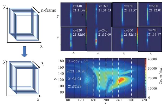
Fig. 1 (top) Original snapshots obtained by HySCAI I ( $y,l$ ), and (bottom) reconstructed image ( $x,y$ ) at 557.7 nm.
