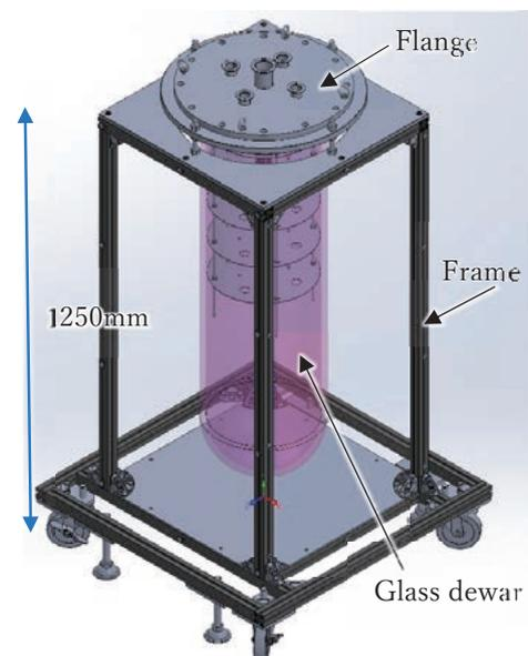
Fig. 10 Assembly drawing of designed flange and frame
