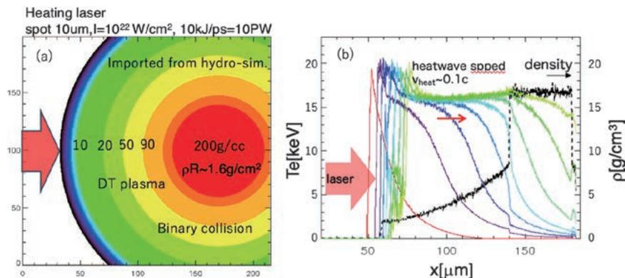
Fig. 2 (a) Initial conditions of the calculation: density profile of the detonation plasma calculated by PINOCO; (b) Time evolution of the bulk-electron temperature on the laser axis (0.5 ps intervals). Propagation of thermal waves.
