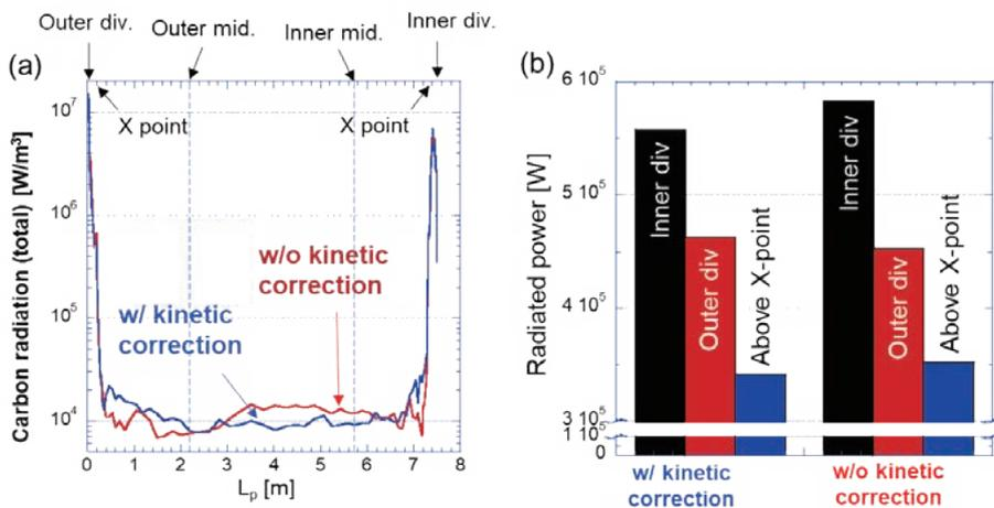
Fig. 4 (a) Impurity radiation profiles along magnetic flux tubes 1 mm outside the separatrix with (blue) and without (red) kinetic correction. (b) Impurity radiation power integrated over the inner, outer, and the main SOL (above the X-point) with and without the kinetic correction.
