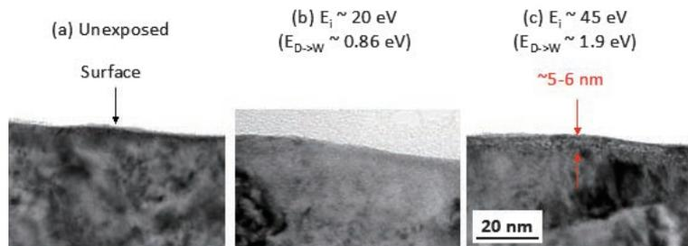
Fig. 1 TEM images of the Deuterium Supersaturated Surface Layer (DSSL). [D. Nishijima *et al.*, Nucl. Fusion **63**, 126003] (2023).
