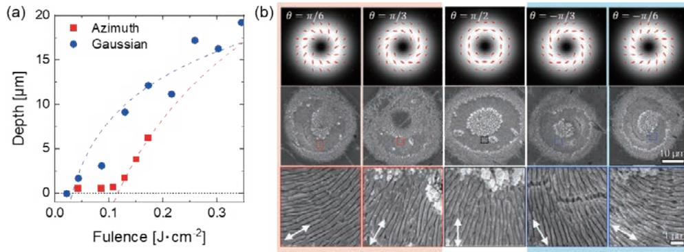
Fig. 6 (a) Dependence of ablation depth  $D$  on laser fluence in the laser irradiation to tungsten surface, (b) Fabricated chiral surface structures employing vector vortex laser. by H. Kawaguchi. (Figure adapted from “Opt. Mater. Express **14**, 424–434, 2024”)
