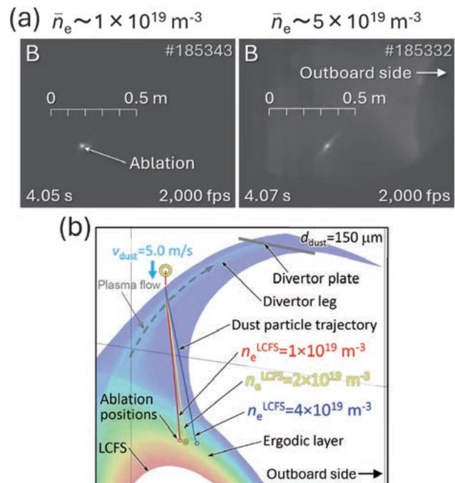
Fig. 1 (a) Images of the ablation of the dropped boron dust particles observed with a fast-framing camera for two different line averaged plasma densities  $\bar{n}_e$  of 1 and  $5 \times 10^{19} \text{ m}^{-3}$ . (b) the simulations of the dropped dust particle trajectories in background plasmas with three different plasma densities at the Last Closed Flux Surface  $n_e^{\text{LCFS}}$  of 1, 2, and  $4 \times 10^{19} \text{ m}^{-3}$ .
