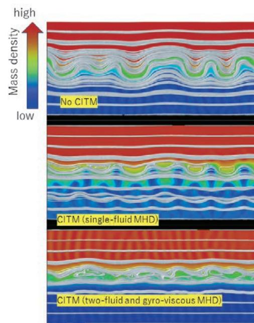
Fig. 5 Mass density (color contours) and 2D magnetic field lines in simulations in which CITM is not observed (top), CITM is observed in a single-fluid MHD simulation (middle), and CITM is deformed by two-fluid and gyro-viscous effects (bottom).
