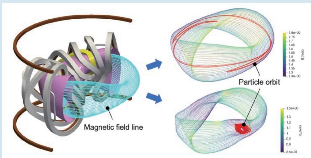
Fig. 1 (Left) the magnetic coils and vacuum vessel of the first conceptual design of a new experimental device (only for a 180° section) and magnetic field line. (Right) typical particle orbit (red curves) in two different magnetic configurations.
