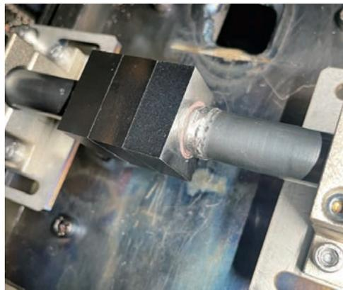
Fig. 2 Experimental set-up for heat loading test in ACT2 facility.
