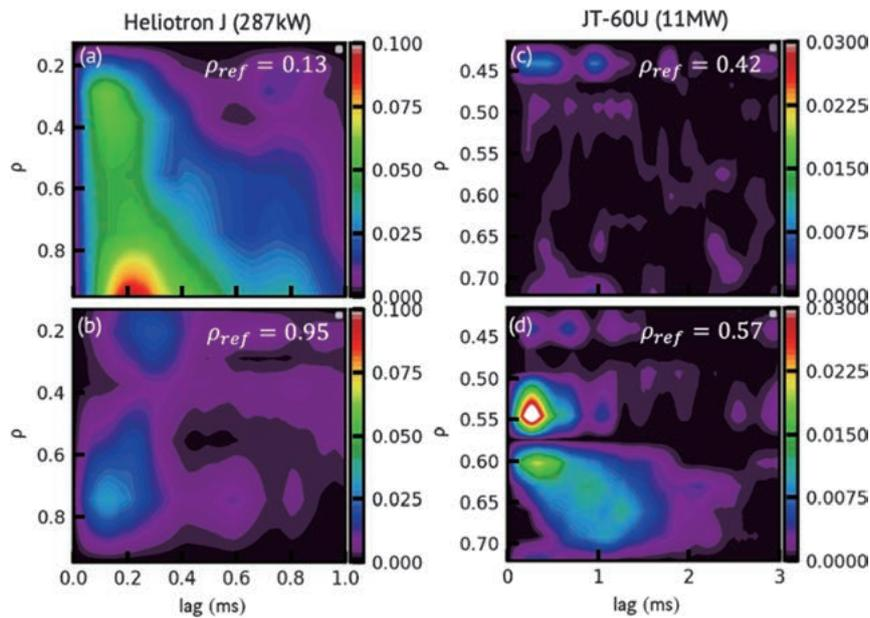
Fig. 1 The transfer entropy of electron temperature fluctuation in (a) and (b) Heliotron J and (c) and (d) JT-60U. The direction of information flow is represented as a reference location  $\rho_{ref}$ , which is indicating  $T_{\rho_{ref} \rightarrow \rho_{others}}$ . [F. Kin *et al.*, *Nucl. Fusion* **64**, 066023, 2024]
