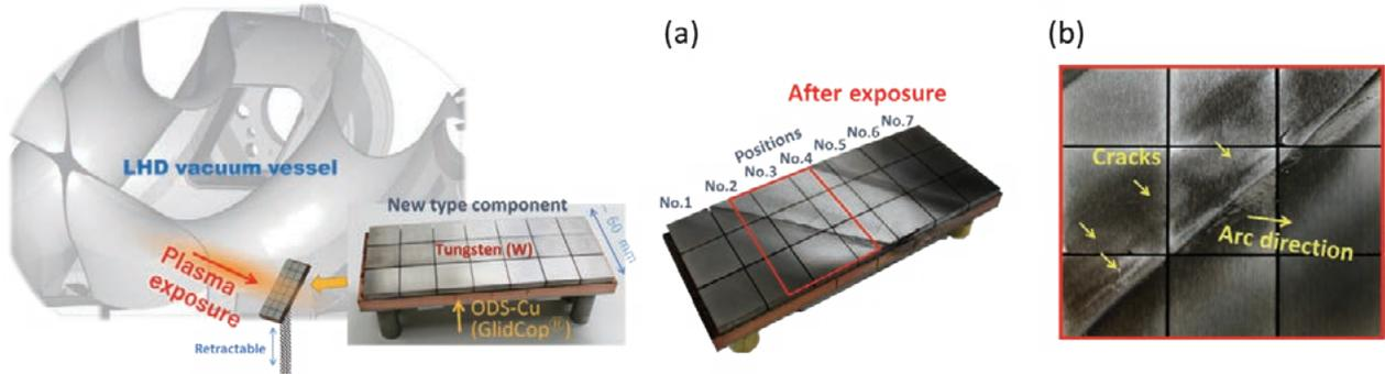
Fig. 3 (left) Schematic view of experimental set-up for irradiation of the new type of divertor heat removal component in LHD. (a) Photograph of the new type of divertor heat removal component after exposure to LHD divertor plasma. (b) Enlarged image of W surface corresponding to red rectangular area of photograph (a).
