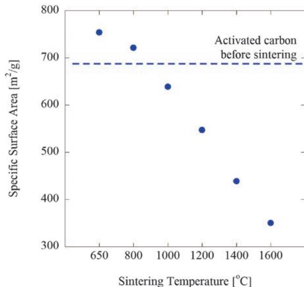
Fig. 3 Specific surface area of activated carbon at each sintering temperature by SPS
