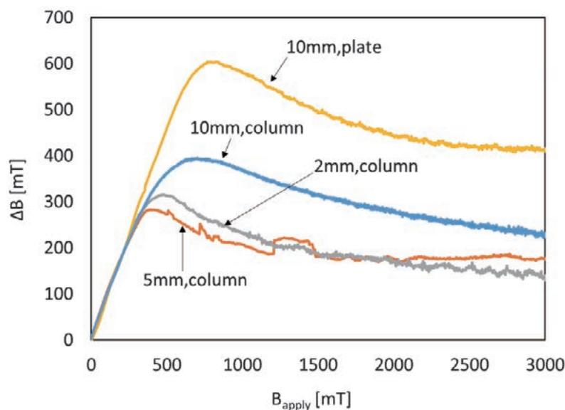
Fig. 1 Magnetic flux density ( $\Delta B$ ) shielded by the plate and column YBCO bulk specimens under the magnetic fields ( $B_{\text{apply}}$ ) at 77 K.
