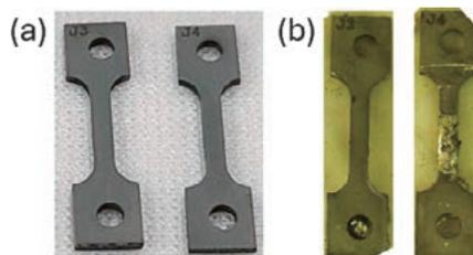
Fig. 5 Optical images of pre-oxidized FeCrAl oxide dispersion strengthened steel (ODS) samples (a) before and (b) after ten days HFIR neutron irradiation (0.8 Fe dpa) in liquid Sn environment at around 460 °C.
