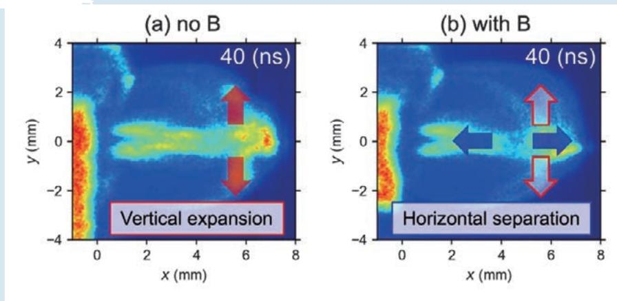
Fig. 1 Self-emission images of the plasma expansion obtained at 40 ns after the irradiation of the drive laser pulse (a) without and (b) with the external magnetic field.
