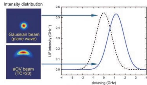
Fig. 1 Beam intensity distributions and numerically obtained LIF spectra in each beam. The figure was made with the data presented in Ref. [1].
