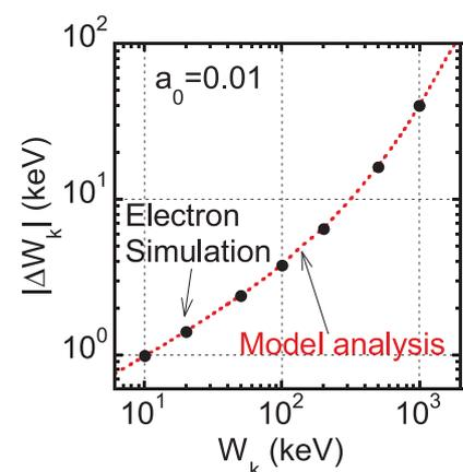
Comparison of the amount of change in electron kinetic energy added, subtracted, or decelerated in a microwave electric field, obtained from model equations and electron acceleration simulations, assuming the initial face of the electric field at the entrance of the electric field area is zero.
