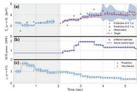
Fig. 1 Results of a control experiment (#186500); (a) control result of  $T_e$  at the plasma center, (b) ECH power adjusted using ASTI, (c) distribution (expected value and one standard deviation) of  $C_e$  at  $\rho = 0.5$  used in the prediction step and filtered.
