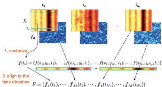
Fig. 2 Procedure of the multi-field SVD for the multi-field data  $F$  [2].
