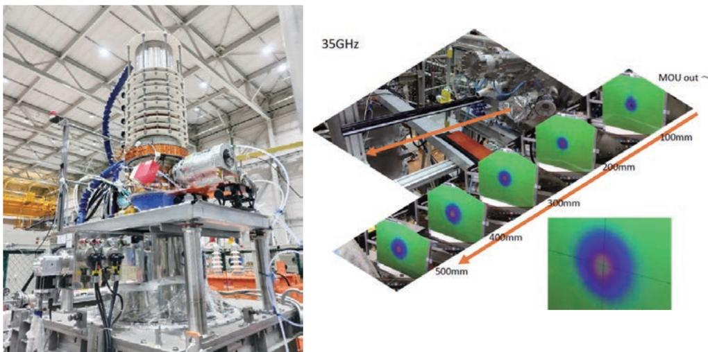
Fig. 2 A dual frequency gyrotron installed for oscillation and transmission testing (left figure). Output beam after passing the MOU. The expected Gaussian beam shape was obtained (right figure).
