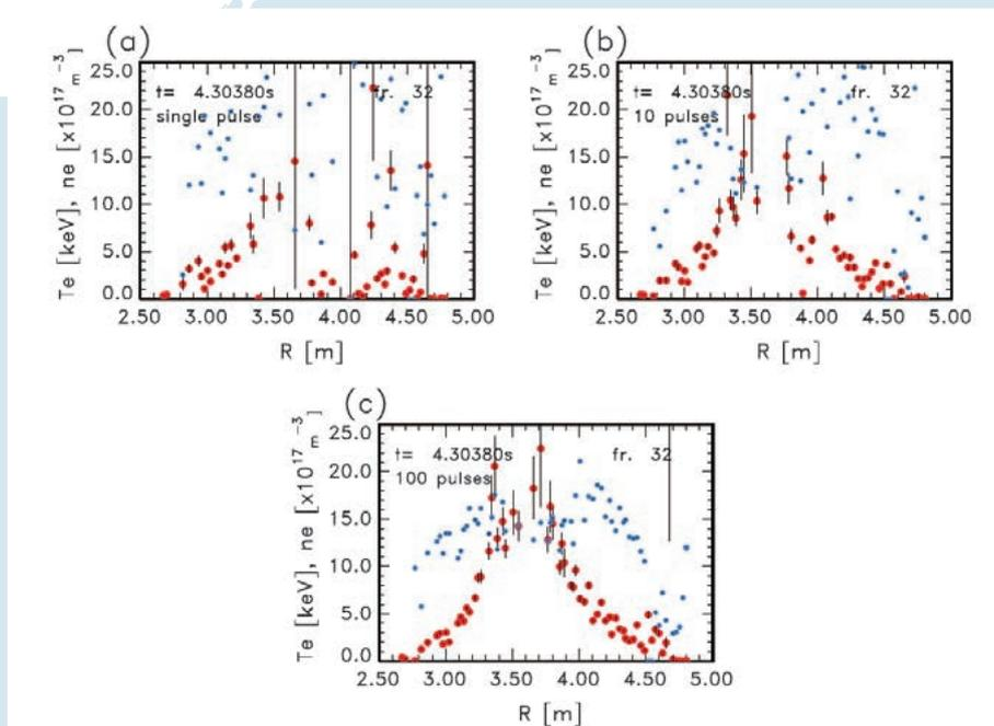
Fig. 1 The red closed circles show the  $T_e$  profile and the blue closed circles show the  $n_e$  profile. (a) Data by a single laser pulse is used. (b) Signals of ten laser pulses are averaged. (c) Signals of 100 laser pulses are averaged. [1]
