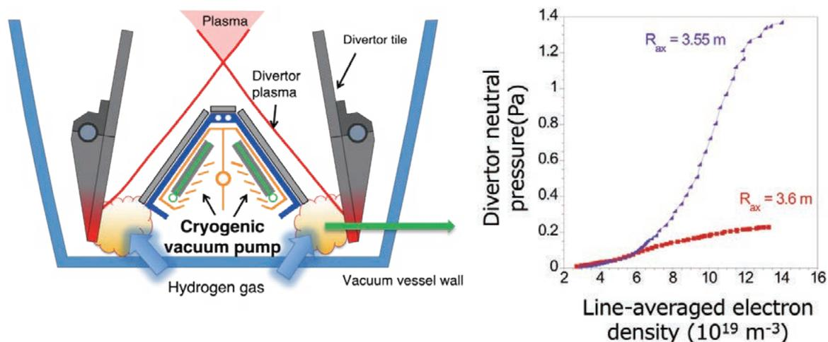
Fig. 2 At the edge of the plasma confined by the magnetic field in the Large Helical Device (LHD), the plasma is drawn into a region called the divertor system, where the plasma becomes neutral gas. In this achievement, a very high neutral pressure of 1.4 Pa is achieved in a specific magnetic field configuration.
