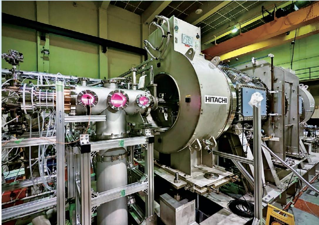
Fig. 1 Picture of the superconducting mirror machine “Pilot GAMMA PDX-SC.”
