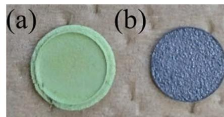
Fig. 6 Optical images of W (a) and W-10%Re alloy (b) after oxidation in Ar-20%O<sub>2</sub> mixture gas at 1073 K.
