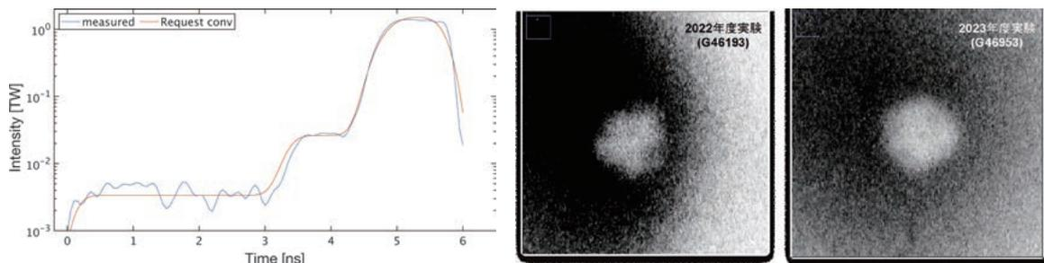
Fig. 1 (Left) Three-stage pulses are generated as requested by hydro-simulation. (Right) Backlight images of imploded plasma observed in FY2022 (Middle) and in FY2023 (Left).
