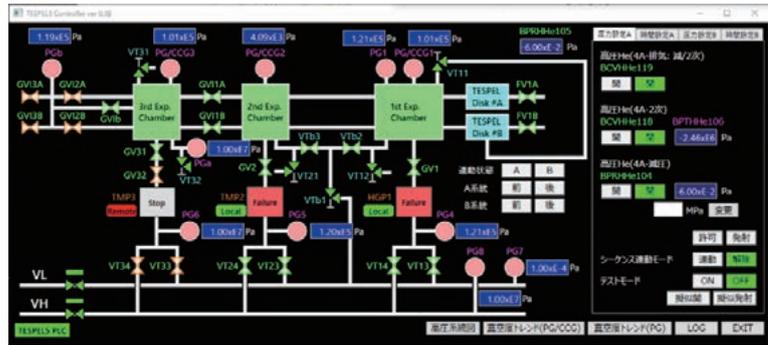
Fig. 11 TESPEL remote-control software operation view
