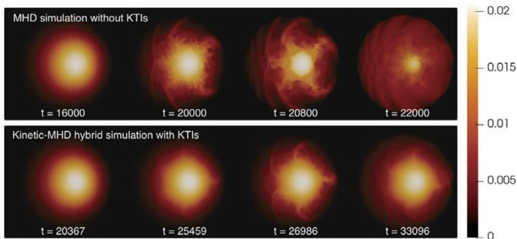
Fig. 2 Time evolution of the pressure profile on a poloidal cross section obtained from the MHD simulation without KTIs (the upper row) and the kinetic-MHD hybrid simulation with KTIs (the lower row) for a resistive infernal mode. Time is normalized by Alfvén time.
