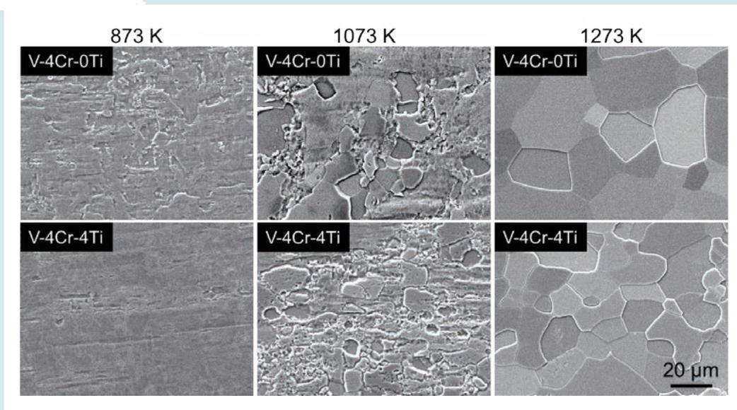
Fig. 1 Scanning electron microscope (SEM) images of cold rolled high-purity vanadium alloys after 873–1273 K annealing for 1 h.
