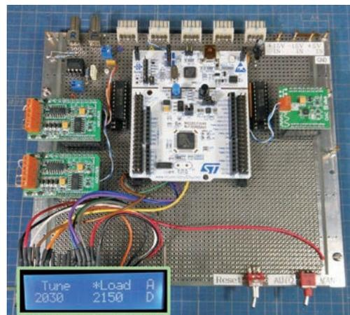
Fig. 5 New control circuit of the impedance matcher for the NBI's RF ion source
