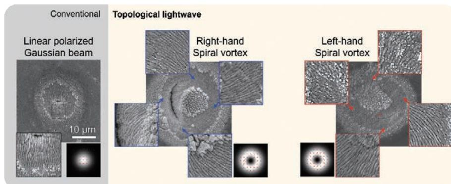
Fig. 1 Topological lightwave laser processing realized arbitrary chiral surface texturing for fusion material (tungsten), provided by H. Kawaguchi. (Reconstructed from Figs. 2 and 4 of “H. Kawaguchi *et al.*, *Opt. Mater. Express* **14**, 424–434, 2024”).
