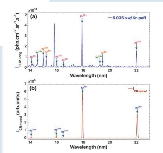
Fig. 1 (a) Experimental extreme ultraviolet spectrum of highly-charged Kr ions (14–23 nm) in the LHD, (b) comparative synthetic  $\text{Kr}^{25+}$  spectrum from the CR model
