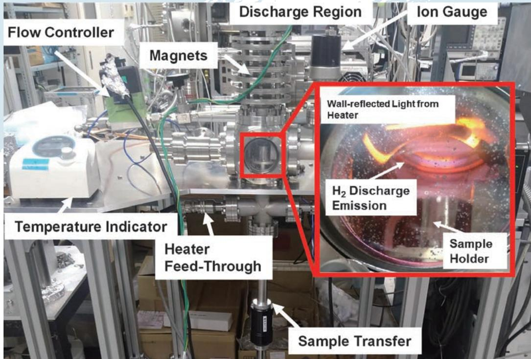
Fig. 1 Newly constructed compact plasma device to be installed in a radiation-controlled area for measurements of tritium retention and distribution in liquid and solid Sn.
