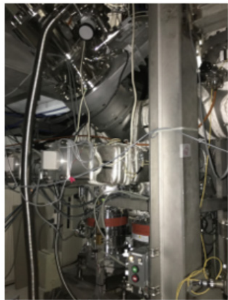
Fig. 6-4 Picture of vacuum pumping system for CHS
