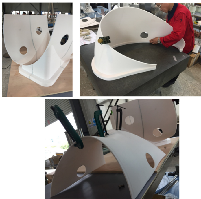
Fig. 4.3.4-3 Pictures of assembled real scale 3D vacuum chamber model made by 3D printer.
