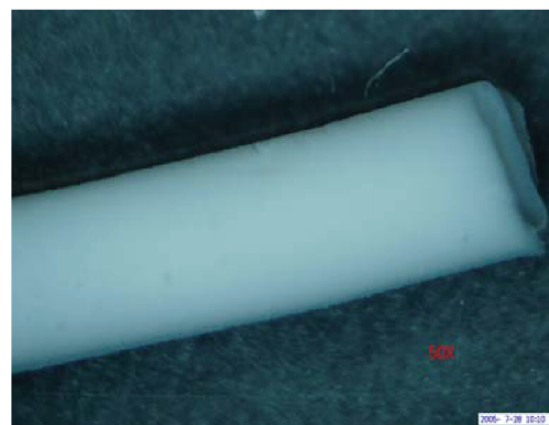
Fig2. the morphologies of UHMW-PE foams, 5.8\text{mg/cm}^3
