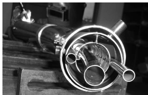
Fig.2. Inner vessel cryopump under outer target of low divertor in EAST
