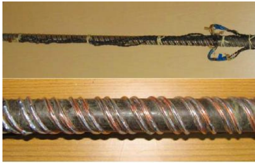
Fig. 5. Photos of the helical wiggler coil
