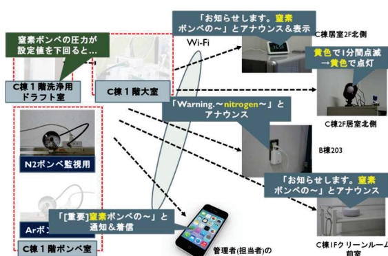
Fig.4: Notification when the pressure of the nitrogen cylinder drops
