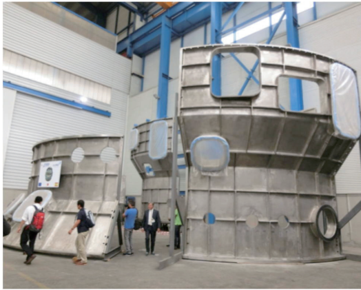
Fig. 3 Cryostat vessel body cylindrical section under fabrication in Spain.
