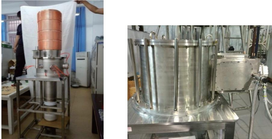
Fig.2 (a) short pulse 1MW gyrotron (b) superconducting magnet
