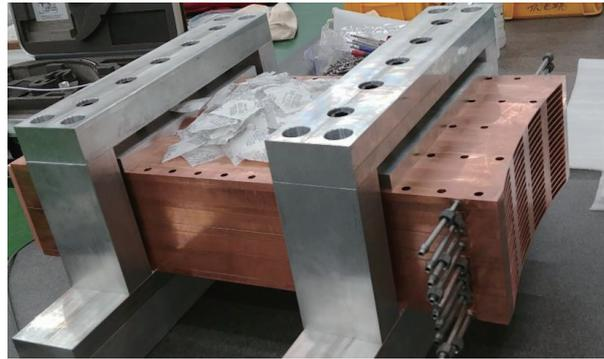
Fig. 4 The photo of finished PAM. Launcher mouth were shaped along the plasma curvature.
