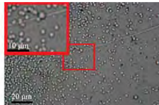
Fig. 6 Optical microscope image of etch pits for group ① in Fig.5 after etching time of 120 min
