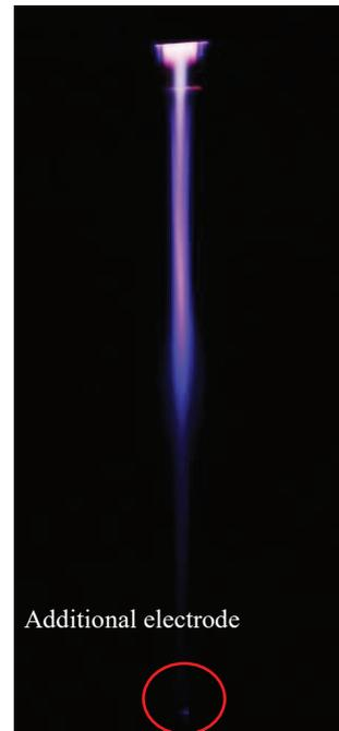
Fig. 7: Digital image of the APPJ with an additional electrode
