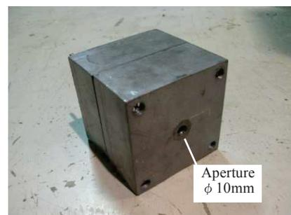
Fig. 3 Appearance of X-ray detecting device
