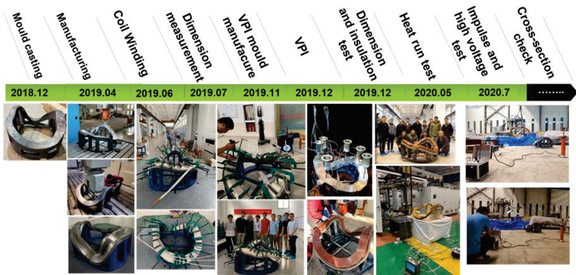
Fig. 5.4.2 The main manufacture points of the MC4 mockup coil.
