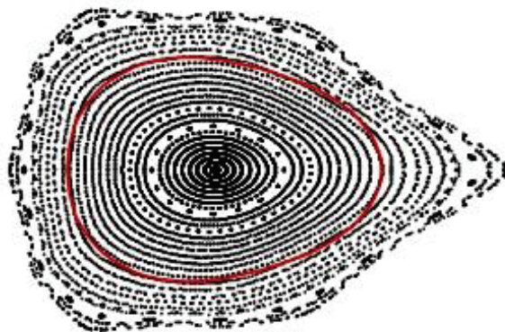
Fig. 3.10-2 Punctual plots of magnetic surfaces for CFQS configuration produced by 16 modular coils. Red line corresponds to the LCFS of the 3rd plot in Fig. 3.10-1.
