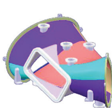
Fig 2.3-1 Material pieces divided plan for vacuum vessel type A. It will be reviewed in the detailed design.
