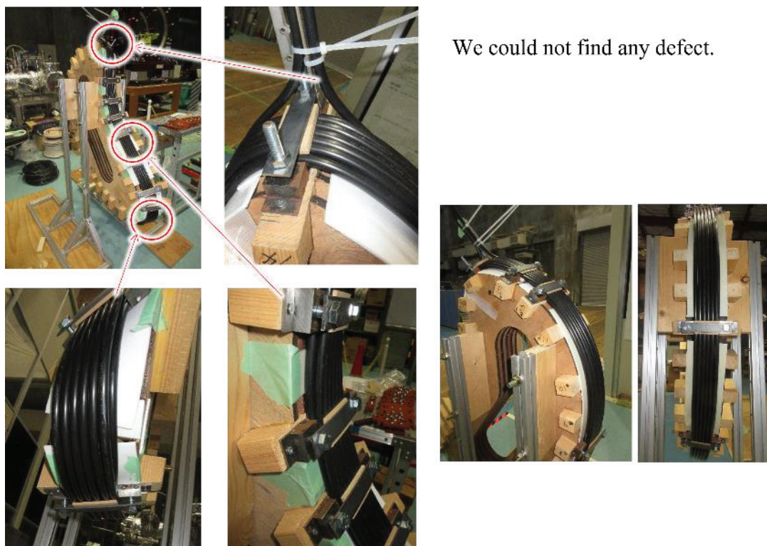
Fig 4.1-12 Visual check after winding the cable. We could not find any defect.
