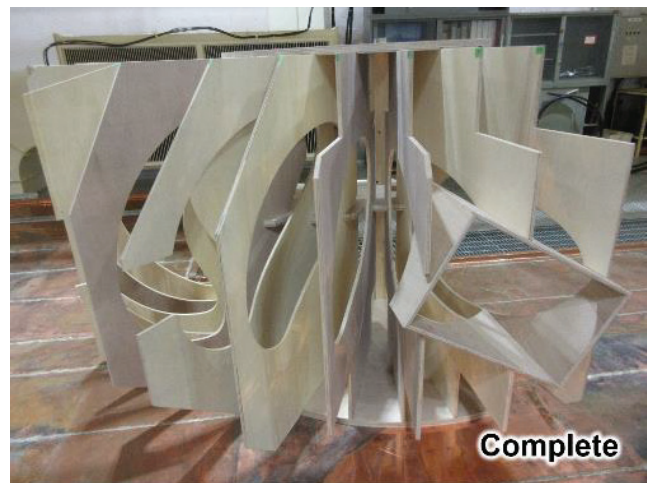
Fig 4.2-2 All parts for a model were assembled in NIFS. Each of 24 parts was made by wood processing company.
