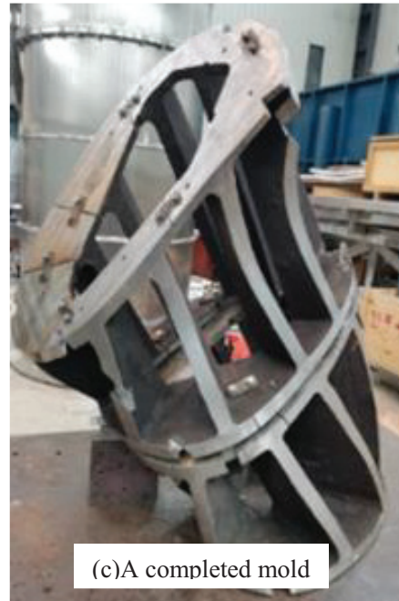
Fig 2.2-2 Mold for thin plats assembly and welding by the CNC machining.
