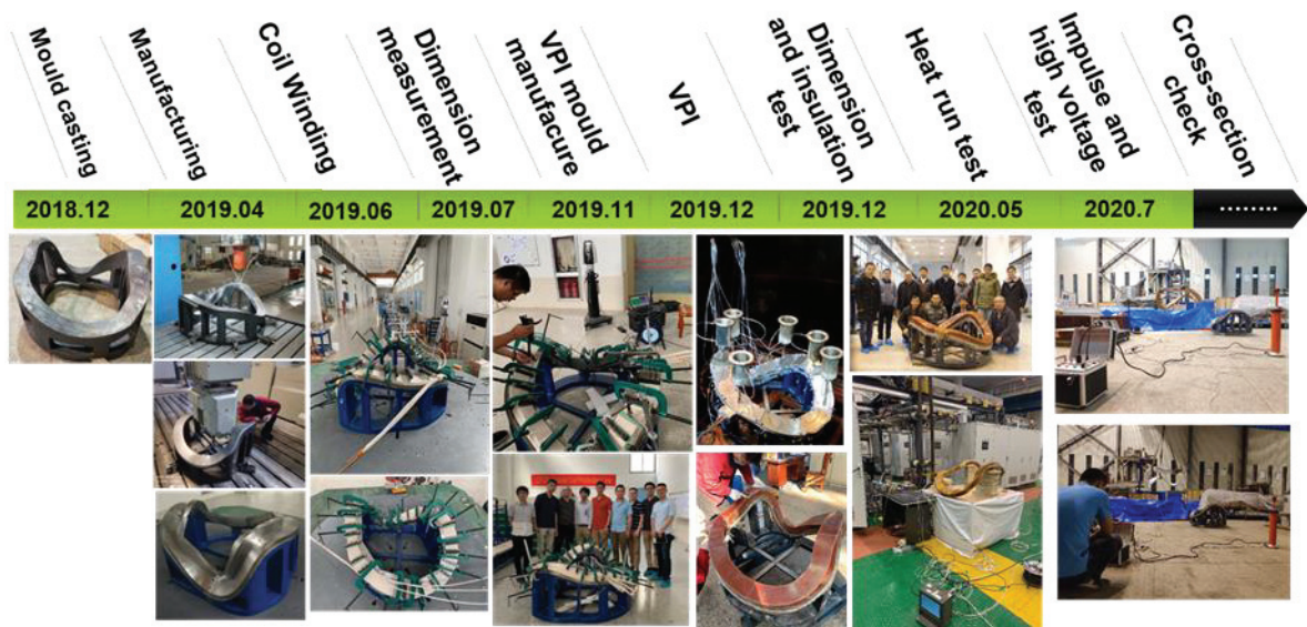
Fig 1.5-2 The main production points of the MC4 mockup coil.
