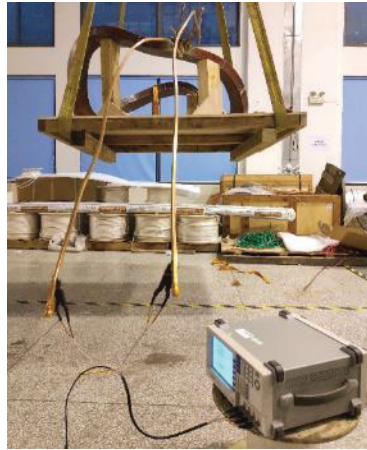
Fig 1.8-2 Scene of the inductance measurement. To reduce the influence of the magnetic material under the floor, the whole was floated and measured.
