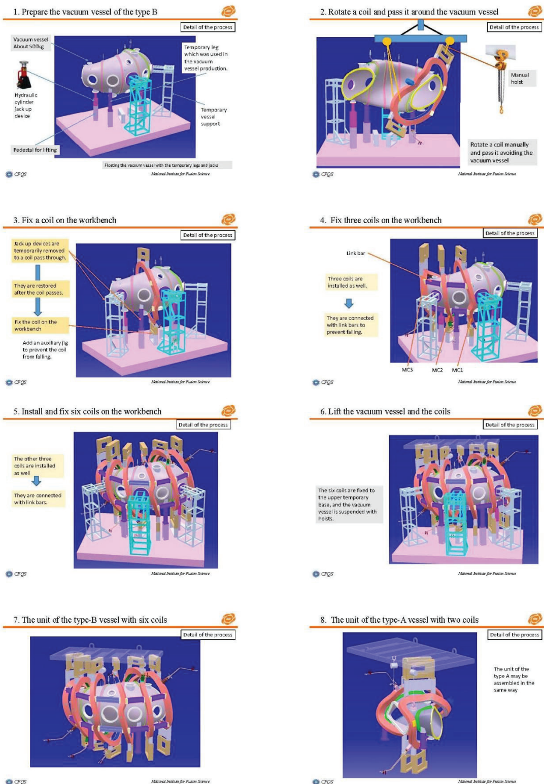
Fig 5.1-1 Pre-assembly process of the modular coil and vacuum vessel.
