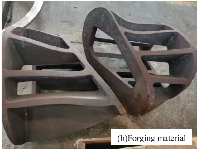
Fig 2.2-2 Mold for thin plats assembly and welding by the CNC machining.
