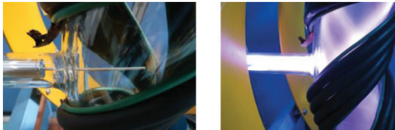
Fig 3.3-2 The Langmuir probe inserted into the vacuum vessel. It is used to estimate the electron temperature and electron density. The left picture shows the tip of the probe and right shows the plasma around the probe.
