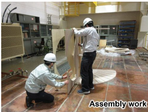
Fig 4.2-2 All parts for a model were assembled in NIFS. Each of 24 parts was made by wood processing company.
