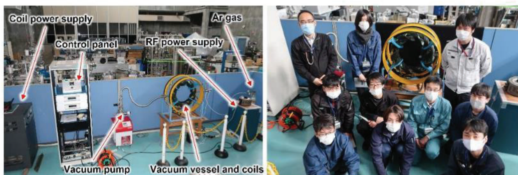
Fig 3.1-2 Redevelopment of the SSHD at NIFS. The SSHD was transferred to NIFS in 2019 for the purpose of training technical staff on the handling of plasma equipment.
