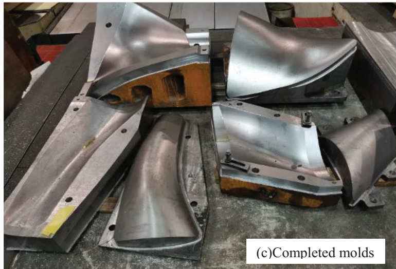
Fig 2.2-1 Pressing die made by the CNC machine.
