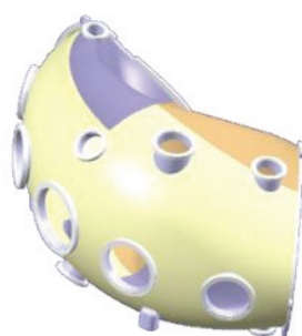
Fig 2.3-2 Material pieces divided plan for vacuum vessel type B. It will be reviewed in the detailed design.
