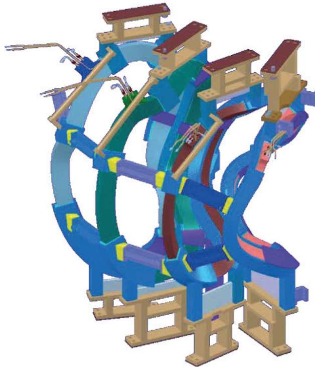
Fig 4.2.2-5 Modular coil system with the PLCL, showing coils, legs, coil cases as a supporting structure, linked beams between the modular coils and the coil leads.
