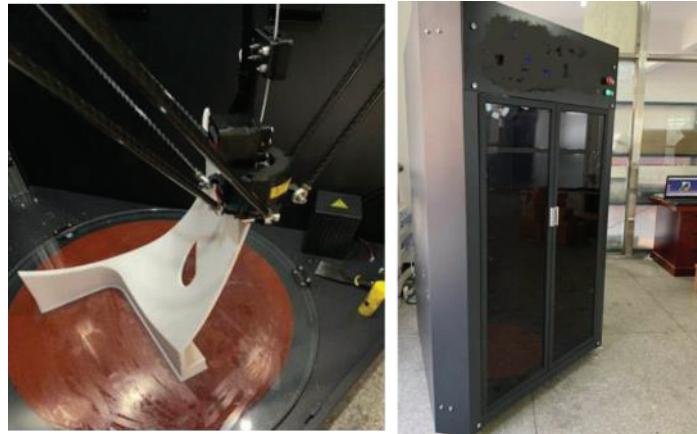
Fig 3.2-5 3D printer to fabricate real scale vacuum vessel model.
