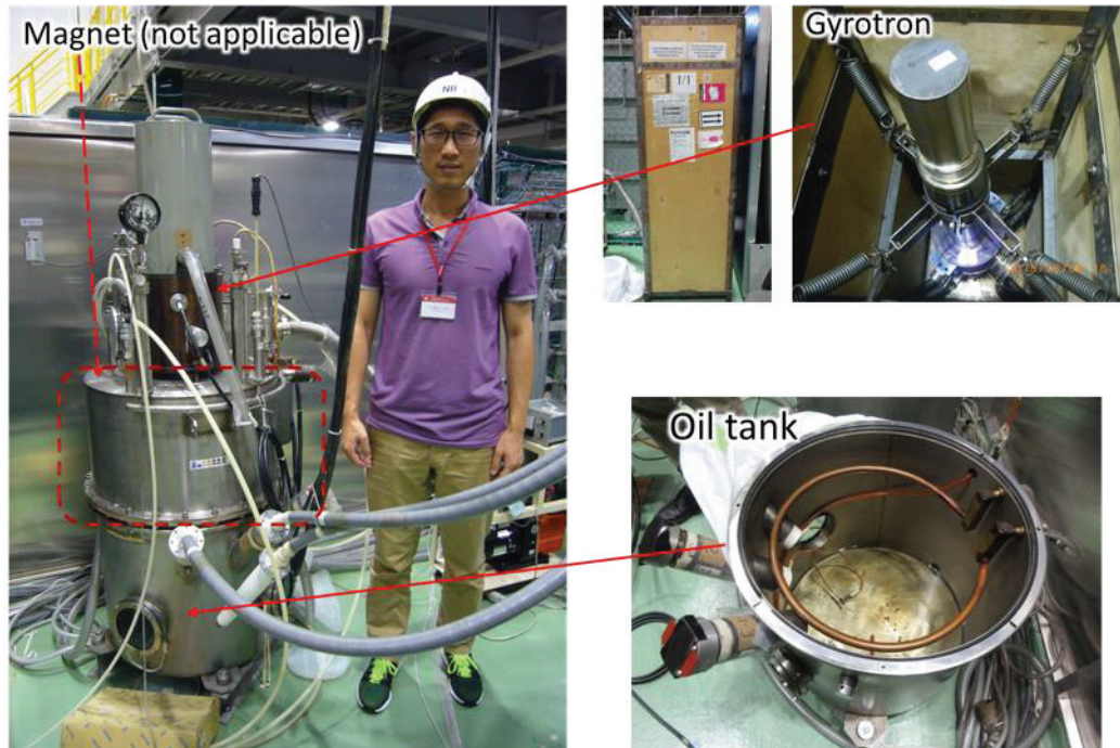
Fig 1.5-2 54.5 GHz gyrotron in the ECRH system for the CHS.
