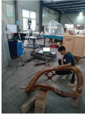
Fig 1.6-3 Scene of the deformation measurement without constraint.
