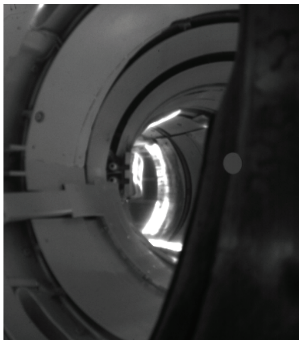
Figure 5 Visible image of the plasma-wall interaction in HT-7 in a disruption event on shot 117750#
