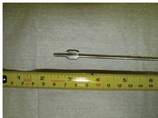
Fig. 3. Photograph of sample stage. The size of stage is around 10 mm × 8 mm. The sheath thermocouple is inserted into the opening of the stage.
