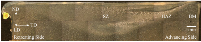
Fig. 1 Cross sectional optical micrograph of friction stir processed ODS-FS
