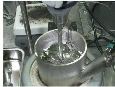
Fig.1. Schematic view and photograph of the HT-UDV measurement of the PbLi flow.
