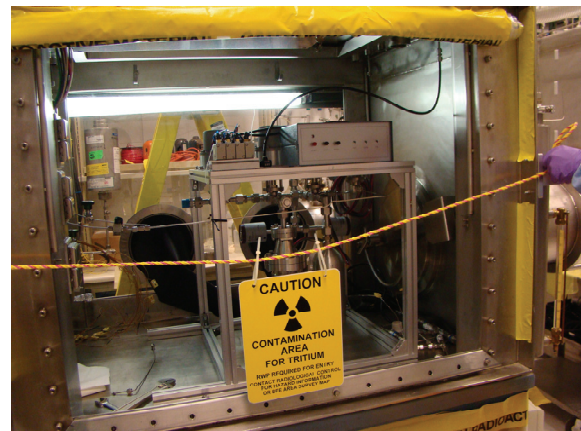
Fig.2 Apparatus for the LiPb-hydrogen isotherm measurement installed in the glovebox of STAR in INL.
