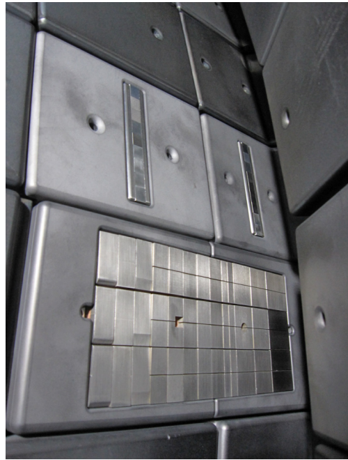
Figure 1. Long term samples installed at KSTAR.
